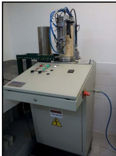
FIGURE 3: Photo equipment developed for readings of volumetric expansion (robot).
