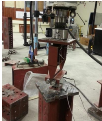
FIGURE 3: WEDGE SPLITTING SETUP ON THE INSTRON MTM.
