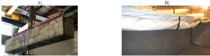
FIGURE 2: A. Concrete slab transported to the temperature-controlled room. B. Large tarp used to maintain high humidity conditions surrounding the slab.
