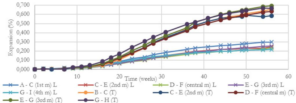
FIGURE 6: Longitudinal (L) and Transversal (T) expansions on the top face of slab 2-R3. For example, the value given for A-C (1st m) L is the average of the longitudinal measurements obtained for columns A through C on the top face (Figure 4).
