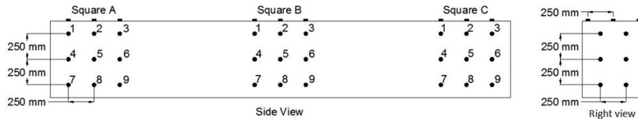
FIGURE 3: Studs locations for the expansion monitoring for the first set of slabs.
