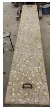
FIGURE 12: Cracking on the upper surface of slab 2-R3 highlighted with black marker.
