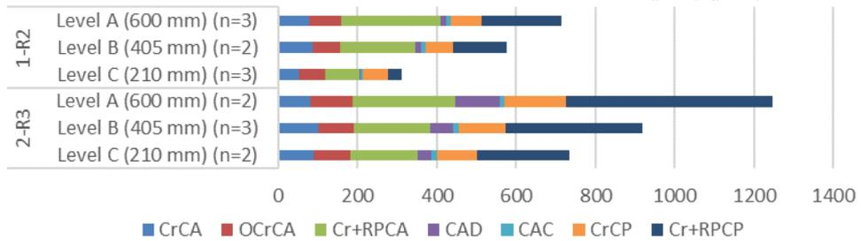
FIGURE 9: Damage Rating Index results for each height in both reactive slabs. The explanation for the abbreviations can be found in TABLE 2 while  $n$  is the number of cores tested.
