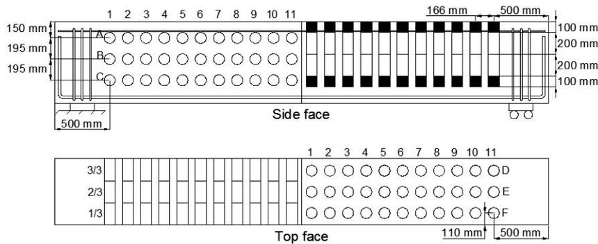
FIGURE 5: Coring plans for slabs 1-R2 and 2-R3. The test results reported in this paper are for cores extracted horizontally, i.e. corresponding to the left portion of the sketches above.
