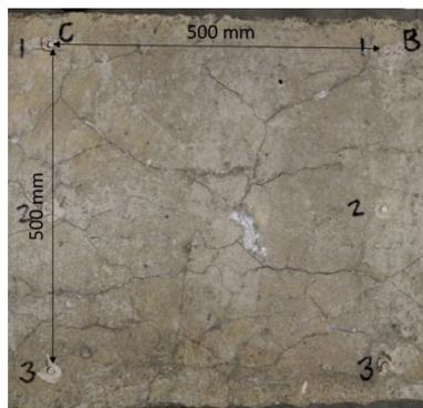
FIGURE 11: Typical cracking present on the top face of slab 2-R3.
