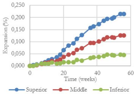
FIGURE 7: Average longitudinal expansions on the side face of slab 2-R3.
