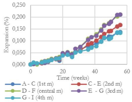
FIGURE 8: Average vertical expansion on the side face of slab 2-R3. For example, the value given for A-C (1<sup>st</sup> m) is the average of the vertical measurements obtained for columns A through C (Figure 4).
