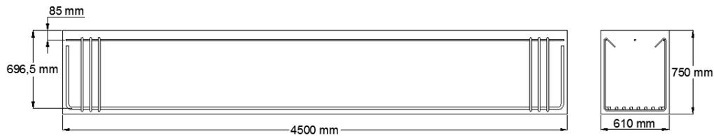
FIGURE 1: Design of the concrete slabs.
