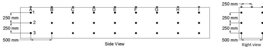
FIGURE 4: Studs location for the expansion monitoring for the second set of slabs.
