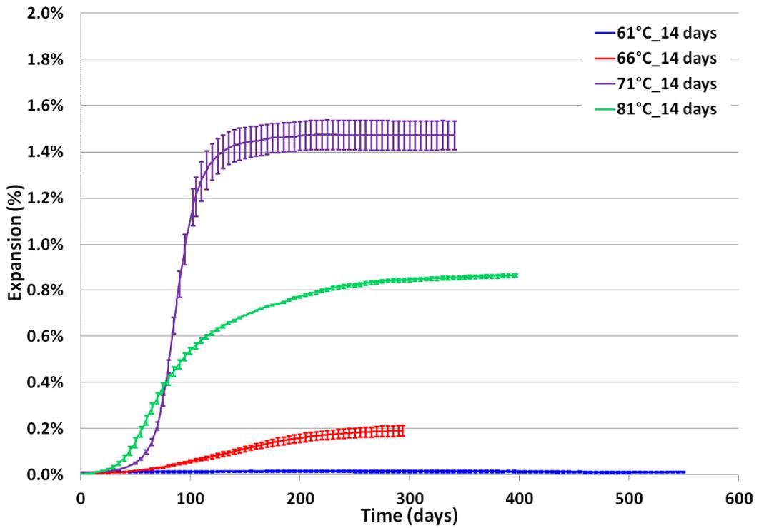
FIGURE 4: Expansion of specimens heated at 61°C, 66°C, 71°C and 81°C during 14 days.
