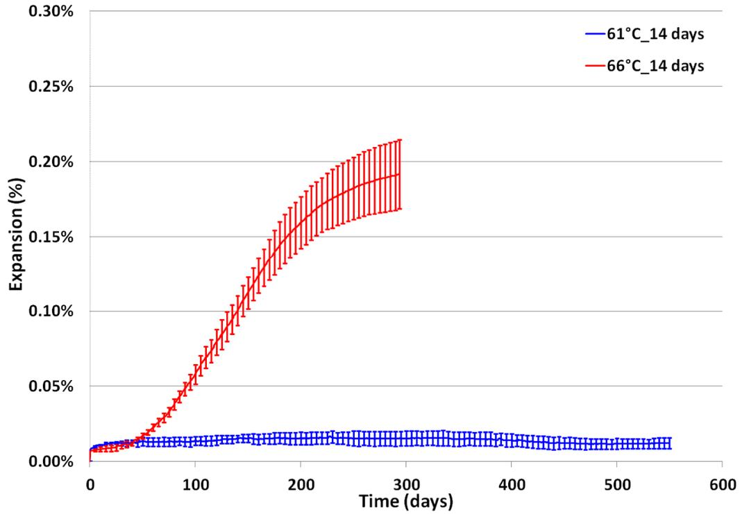
FIGURE 3: Expansion of specimens heated at 61°C and 66°C during 14 days.
