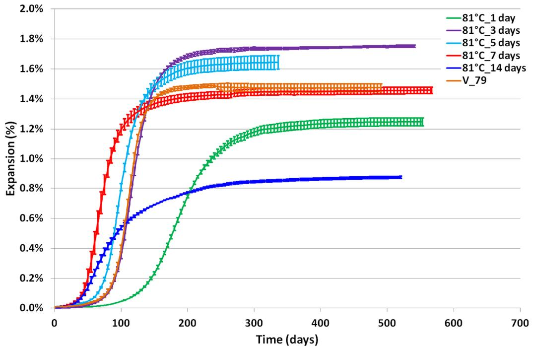
FIGURE 6: Expansion of specimens heated at 81°C during 1, 3, 5, 7 and 14 days.
