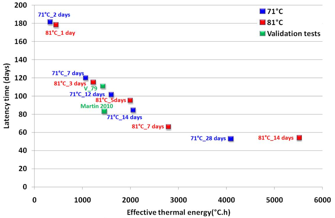
FIGURE 9: Effect of effective thermal energy on latency time.
