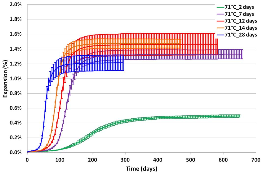
FIGURE 5: Expansion of specimens heated at 71°C during 2, 7, 12, 14 and 28 days.
