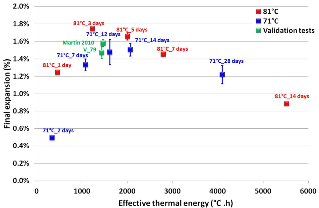
FIGURE 8: Effect of effective thermal energy on magnitude of expansion.
