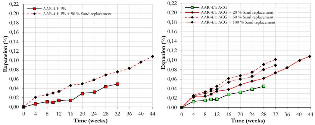
FIGURE 5: Effect of the sand replacement on the ASR expansion.
