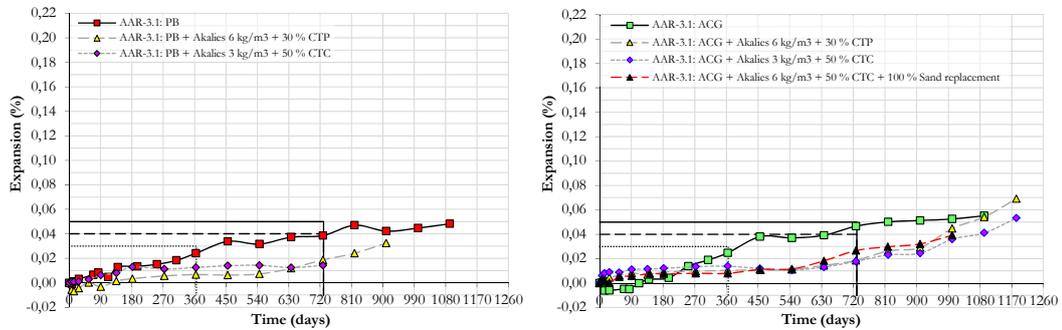
FIGURE 7: Results obtained in the AAR-3 tests.
