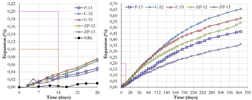
FIGURE 8: Results obtained in the ASTM C1260 test performed to alternative sands.
