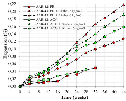
FIGURE 3: Effect of the alkali boosting on ASR expansion (RILEM AAR-4.1 tests).
