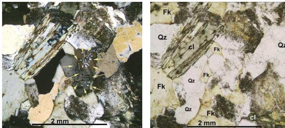
Mineralogical composition, texture and alteration of granite PB; besides quartz (Qz) and potassic feldspars (Fk), biotite transformed in chlorite (cl) is observed. Note the intense alteration of feldspars. The presence of myrmekites can be identified and indicated by the arrows, (in parallel and crossed nicols, on the left and on right respectively).
