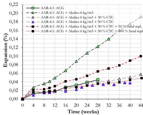
FIGURE 6: Effect of fly ash and sand replacement on the ASR expansion.
