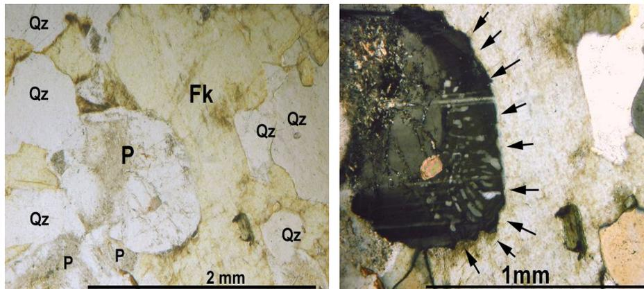
Mineralogical composition, texture and alteration of granite CB; quartz (Qz), plagioclase (P) and potassic feldspars (Fk). Note the presence of myrmekites in the rim of a plagioclase crystal, as indicated by the arrows, (in parallel and crossed nicols, on the left and on right respectively).
