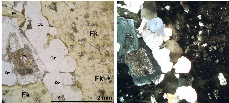
Mineralogical composition and texture of granite ACG; crystal of plagioclase affected by kaolinite alteration (P), quartz (Qz) and potassic feldspar (Fk), (parallel and crossed nicols, on the left and on right)
