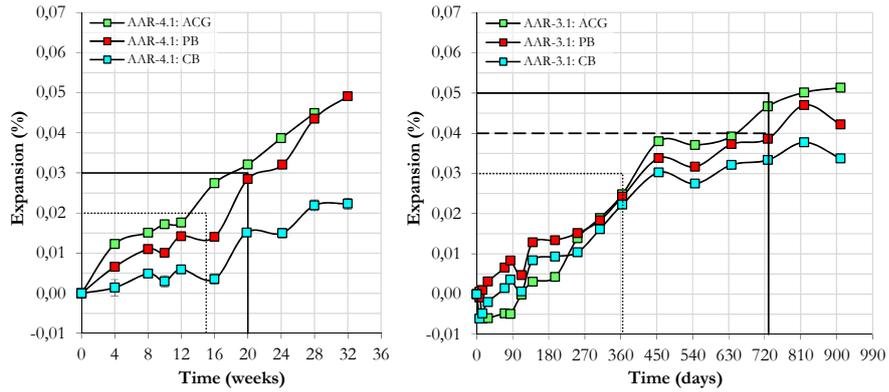
FIGURE 2: Results obtained in the RILEM AAR-4.1 and AAR-3 tests carried out to assess the potential alkali-silica reactivity of the aggregates.
