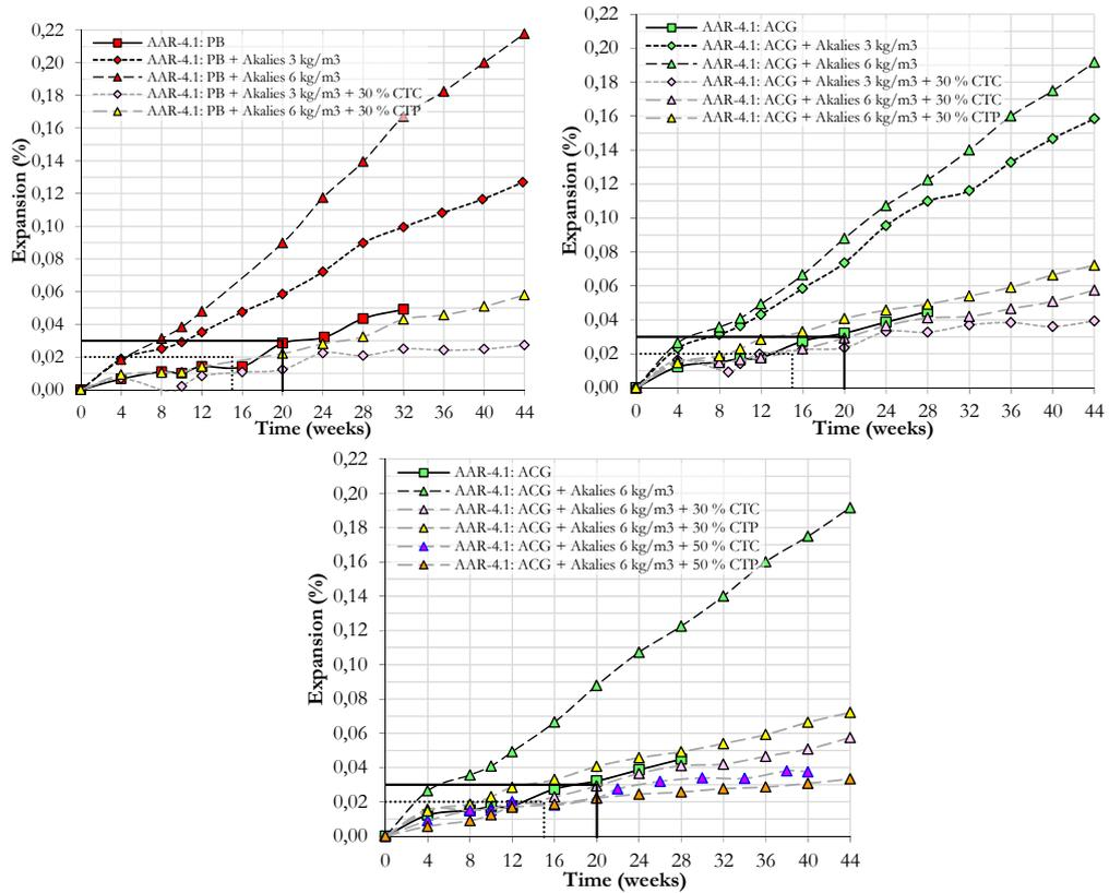
FIGURE 4: Effect of the alkali boosting and fly ash replacement level on ASR expansion.
