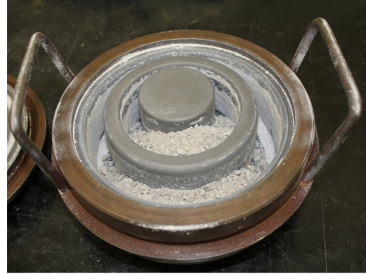
FIGURE 1: A. Set-up used for the hot water alkali extraction using the Espresso method . B. Mechanical tool used to pulverize rock/aggregate materials.
