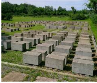
Figure 1: A. CANMET outdoor exposure site. B. Measurements of the exposure blocks.
