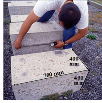
Figure 1: A. CANMET outdoor exposure site. B. Measurements of the exposure blocks.
