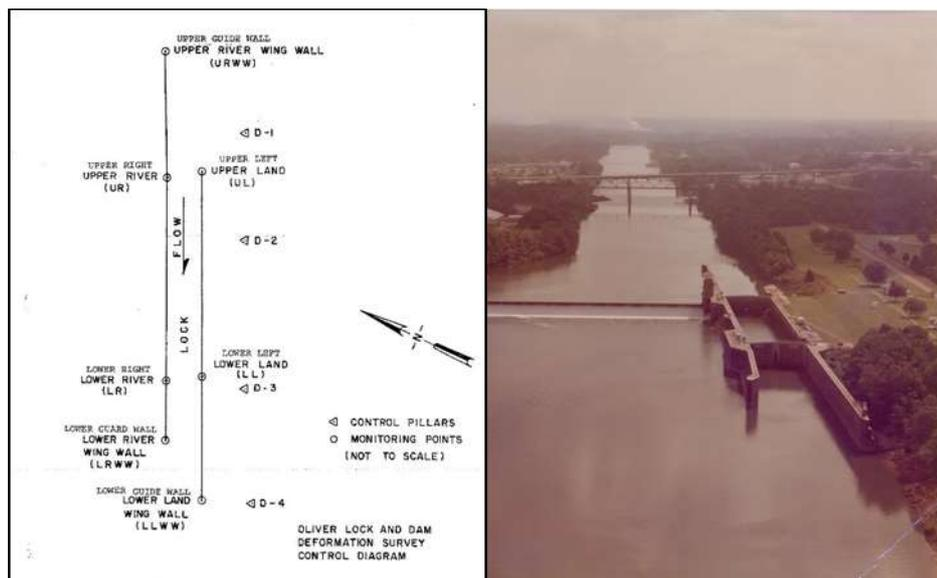
FIGURE 1: Monitoring points and control pillars (left) [3]. View of Black Warrior River and Old Oliver Lock and Dam looking upstream towards Tuscaloosa (right) (photo courtesy USACE Mobile District office).
