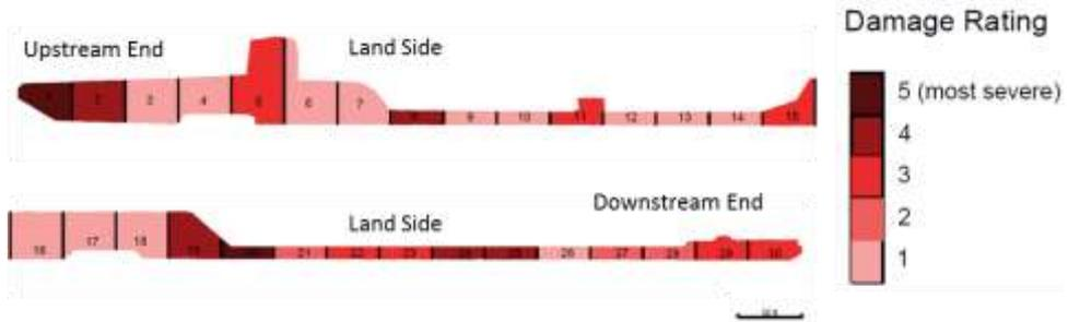
FIGURE 2: Lock schematic with visual survey damage ratings.
