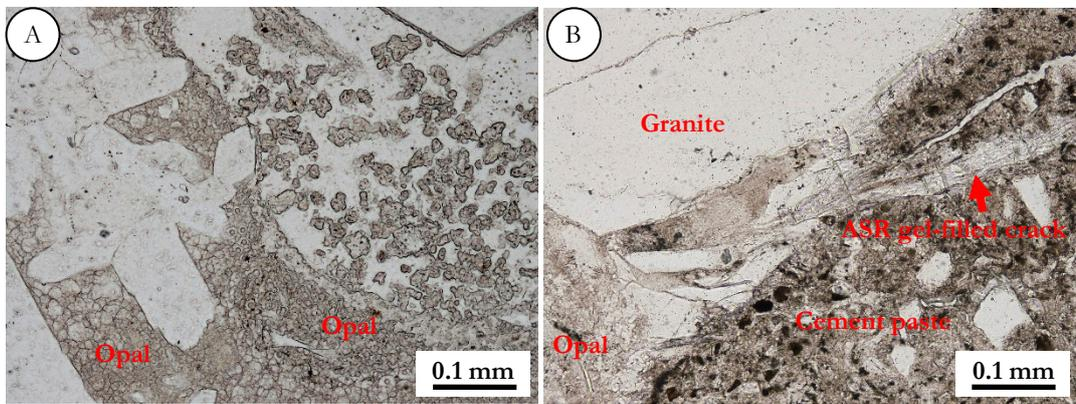
FIGURE 10: A similar ASR case in Southeast Asia under a polarizing microscope (plane polarized light).
