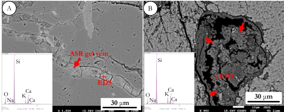
FIGURE 9: SEM-EDS of sand-sized granite.
