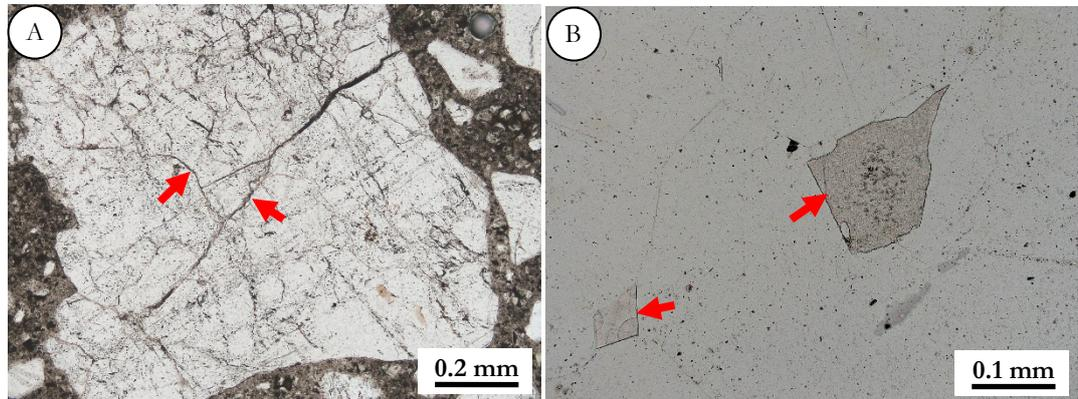
FIGURE 6: Granitic sand under a polarizing microscope (plane polarized light).
