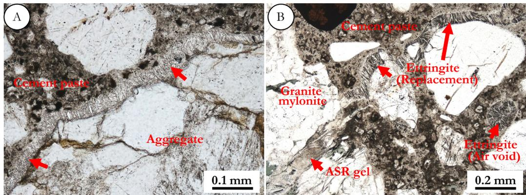
FIGURE 7: Occurrence of ettringite under a polarizing microscope (plane polarized light).
