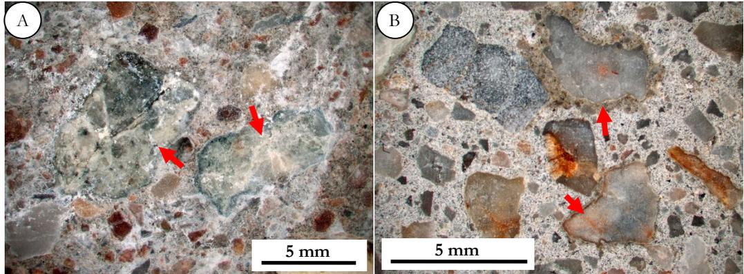
FIGURE 3: Cut surface of concrete. A: Coarse aggregate with crack, ASR gel exudation and reaction rim (Footing A). B: Fine aggregate with ASR gel exudation (Footing D).
