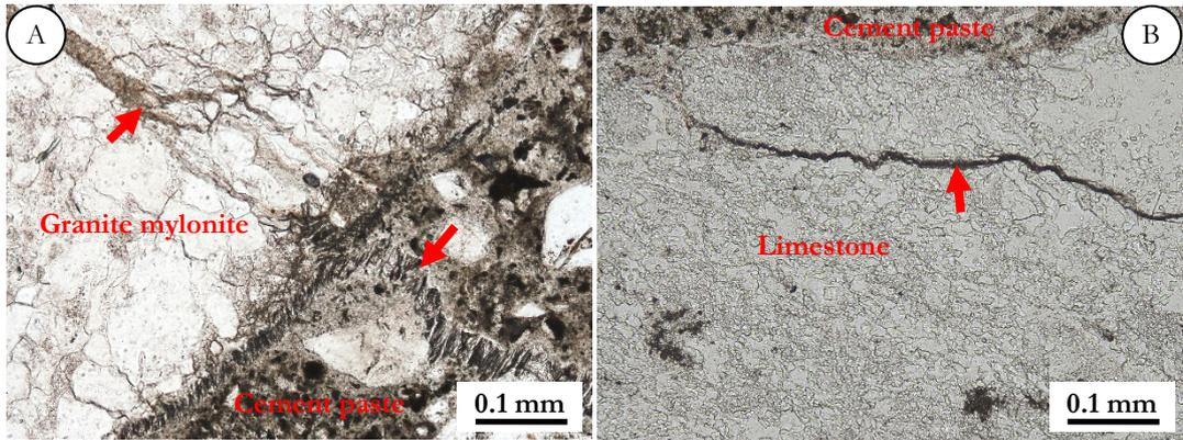
FIGURE 4: Texture of ASR damaged concrete under a polarizing microscope (plane polarized light). A: Granite mylonite (Footing A). B: Limestone (Footing D).
