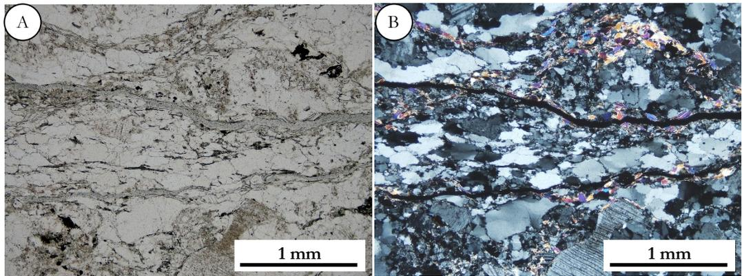
FIGURE 5: Texture of granite mylonite under a polarizing microscope. A: Plane polarized light. B: Crossed polarized light.
