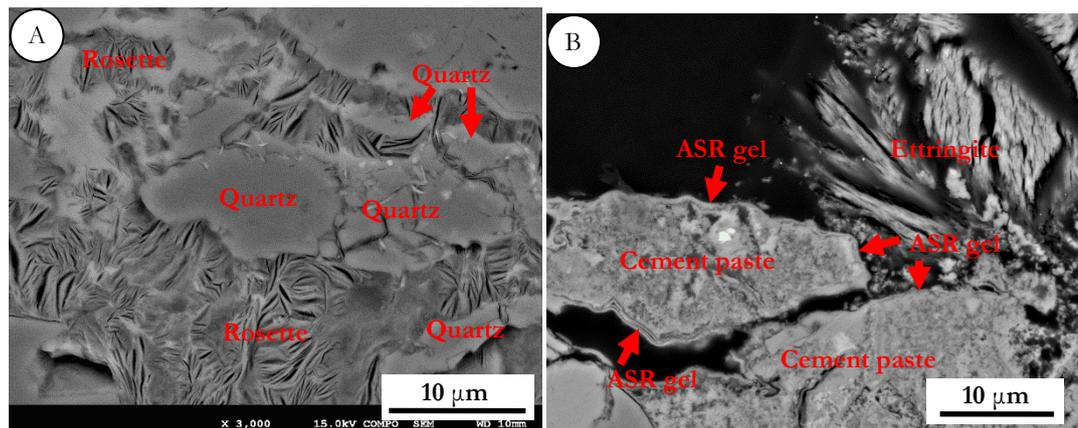
FIGURE 8: SEM photographs. A: ASR gel-filled crack inside granite mylonite (Footing A). B: ASR gel film directly on the crack wall and inner ettringite (Footing A).
