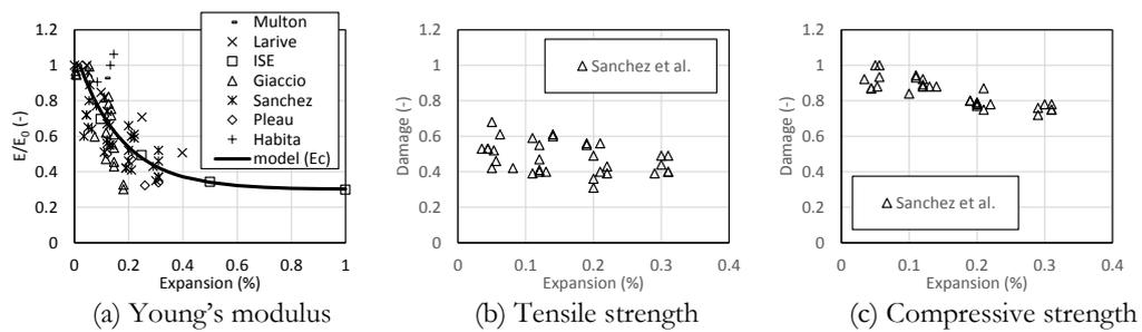
FIGURE 1: Expansion vs. mechanical properties.
