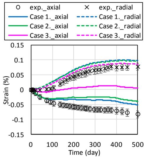
FIGURE 6: Simulated results of concrete subjected to 10 MPa (no steel rings).
