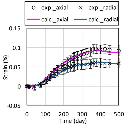
FIGURE 4: Experimental free expansion and calibrated expansion curve by the model.
