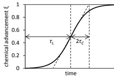
FIGURE 2: Schematic representation of chemical advancement including physical meaning of latency and characteristic times. After [7].
