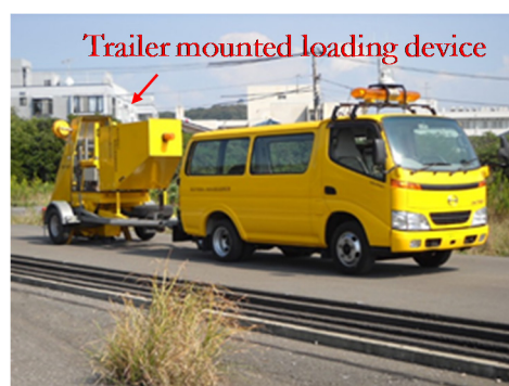
FIGURE 10: Falling weight deflectometer
