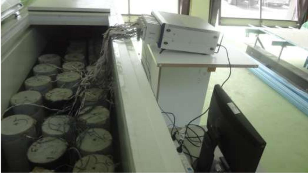
FIGURE 2: Expansion measurement.
