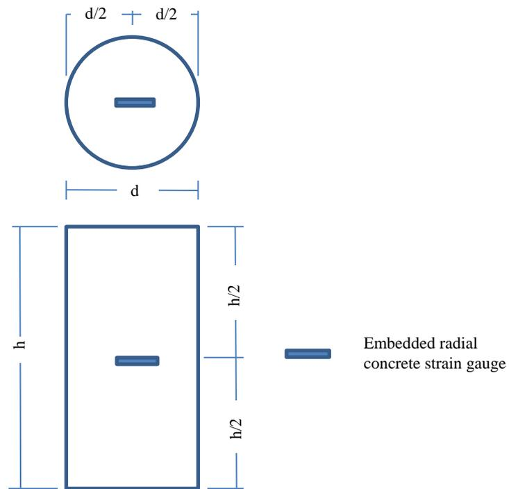
FIGURE 1: Column schematic: position of embedded radial concrete strain gauge.
