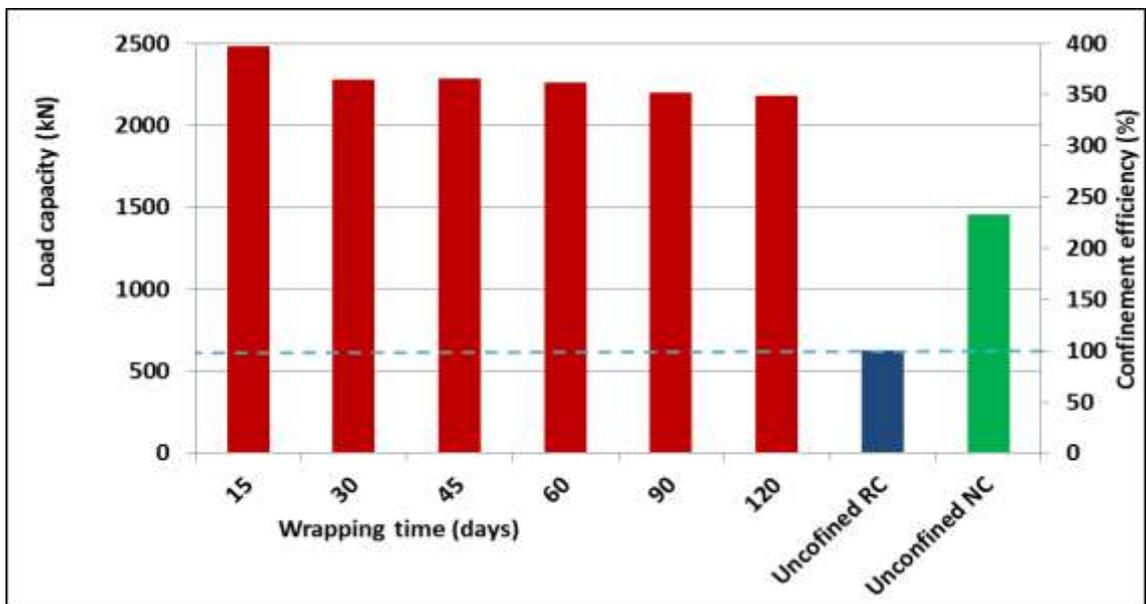
FIGURE 5: 180 days load capacities values for confined affected columns wrapped at different times and unconfined columns.
