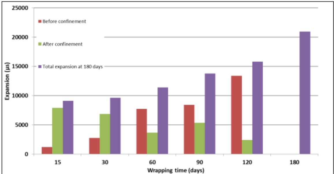
FIGURE 4: 180 days expansion measurement for confined columns wrapped at different times including expansion measurements, before and after confinement.
