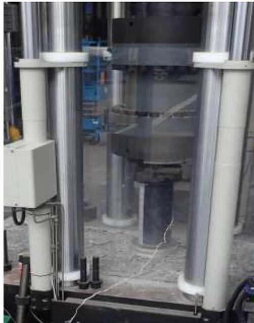
FIGURE 3: Column under compression machine.
