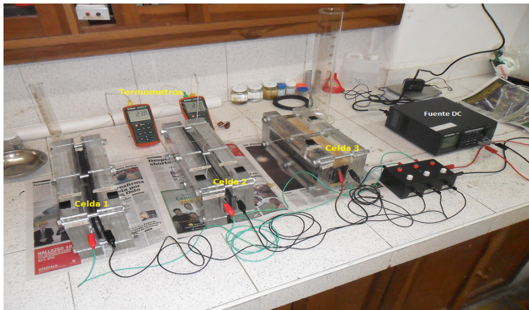
FIGURE 3: Electrochemical impregnation layout during mortar bar treatment (three cells shown).
