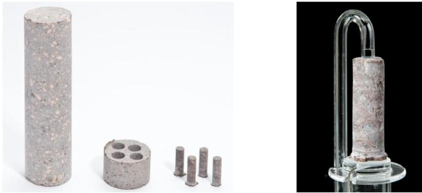
FIGURE 1: Drill core and specimens (left). Cylindrical specimens between push rod and sample table in the analyzer TMA 402 F3 Hyperion Netzsch (right).
