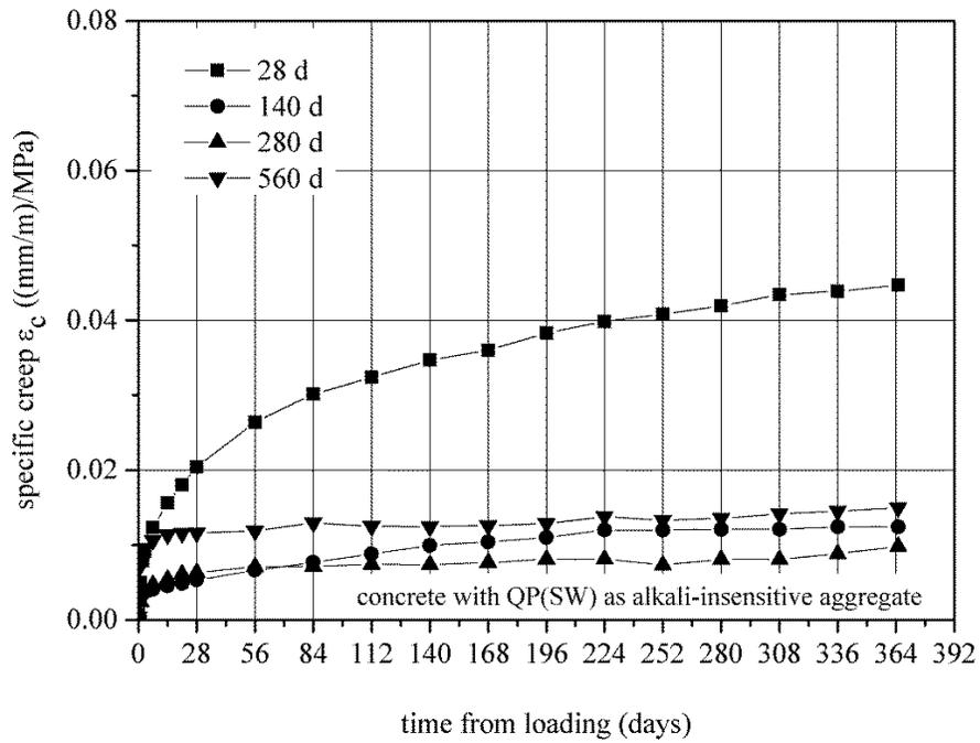
FIGURE 6: Time development of compressive creep of concrete with QP(SW) as alkali-insensitive aggregate, where loading ages are 28 days, 140 days, 280 days and 560 days, relative ambient humidity 80%.
