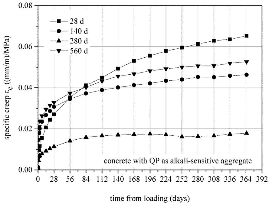
FIGURE 5: Time development of compressive creep of concrete with QP as alkali-sensitive aggregate, where loading ages are 28 days, 140 days, 280 days and 560 days, relative ambient humidity 80%.
