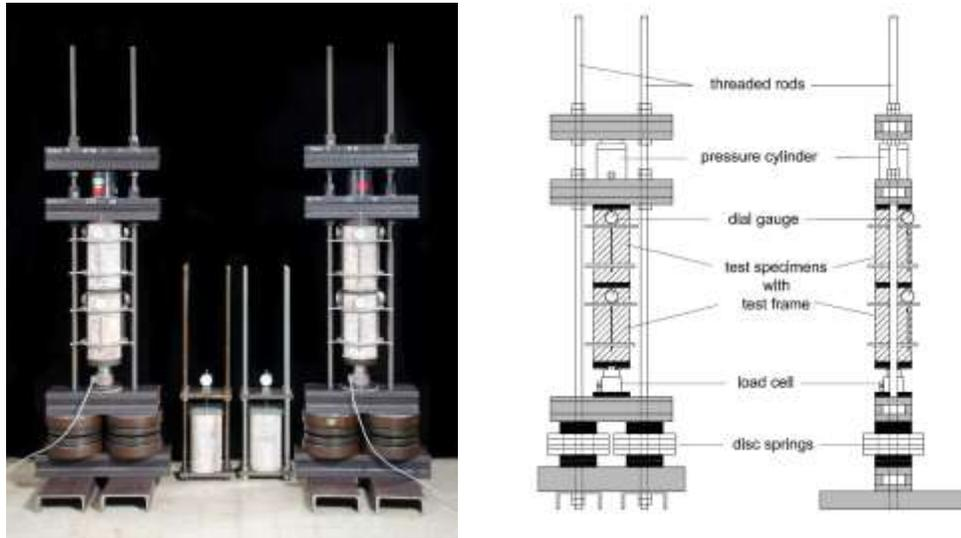
FIGURE 1: Test rig for compressive creep.
