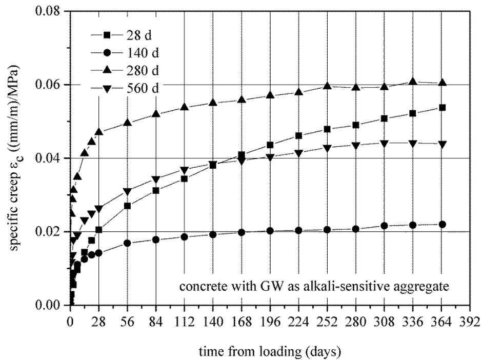
FIGURE 4: Time development of compressive creep of concrete with GW as alkali-sensitive aggregate, where loading ages are 28 days, 140 days, 280 days and 560 days, relative ambient humidity 80%.
