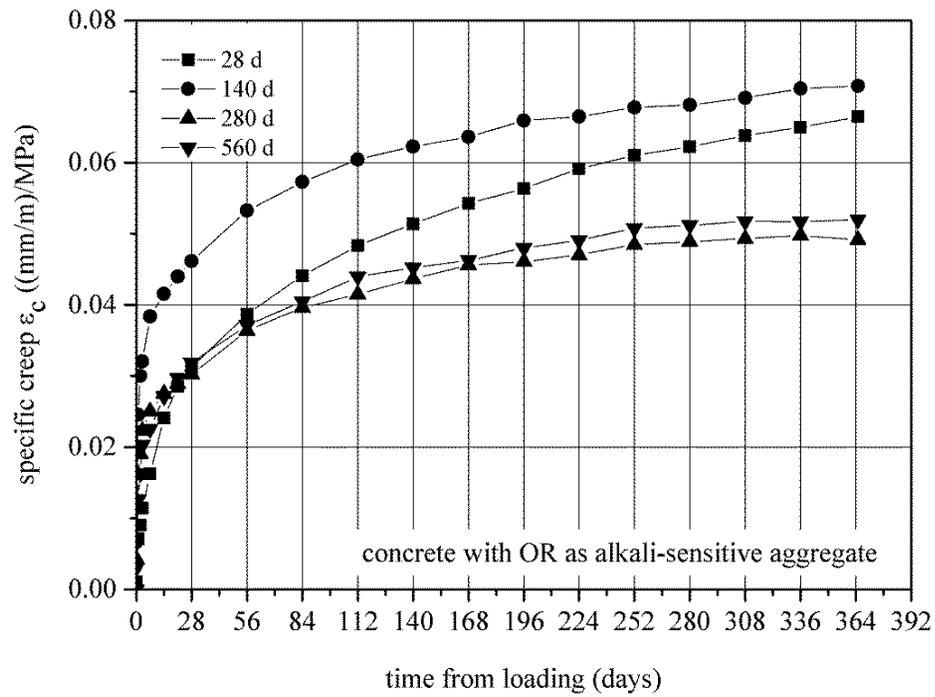
FIGURE 3: Time development of compressive creep of concrete with OR as alkali-sensitive aggregate, where loading ages are 28 days, 140 days, 280 days and 560 days, relative ambient humidity 80%.
