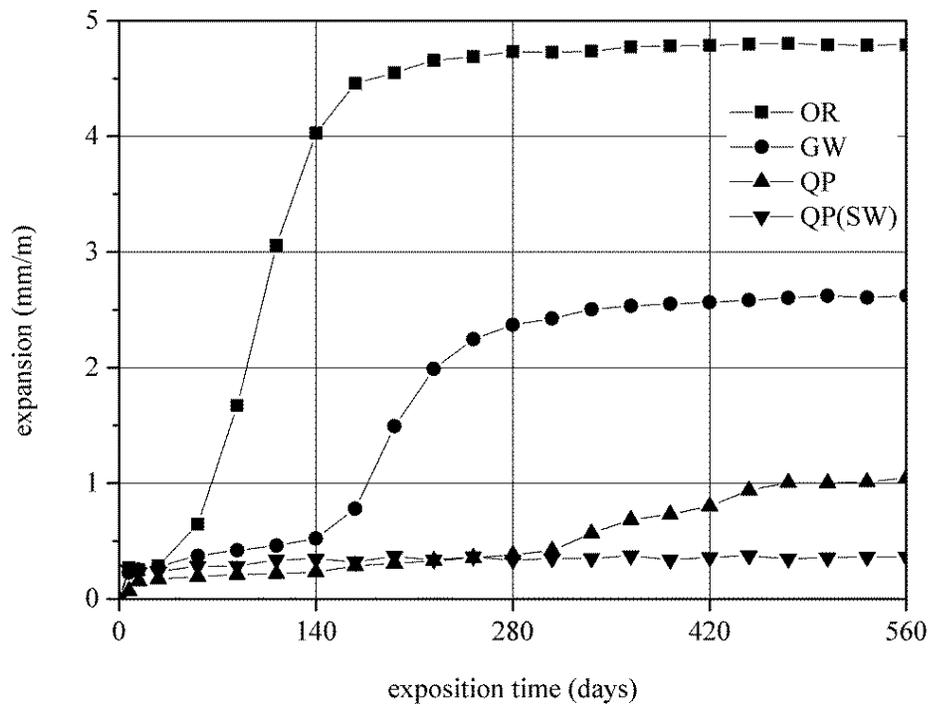
FIGURE 2: Expansion of concrete with OR, GW, QP and QP(SW) as aggregate.
