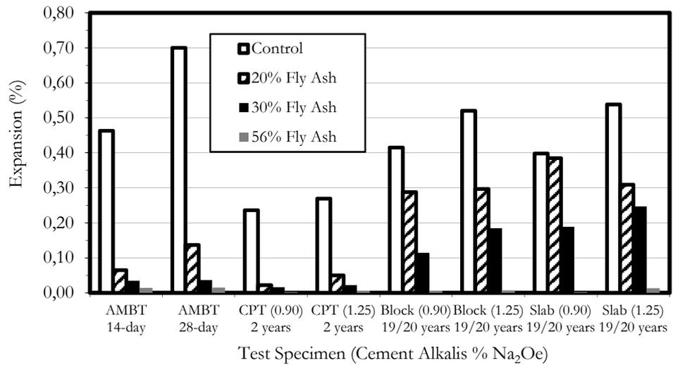
FIGURE 4: CANMET expansion data for Springhill aggregate with a low-CaO (2.06% CaO) fly ash tested in the AMBT, CPT and exposure blocks and slabs.
