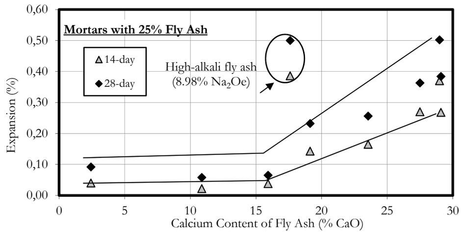
FIGURE 3: Effect of calcium content on expansion of mortar bars containing Springhill aggregate and 25% fly ash (Hayman et al., 2010).
