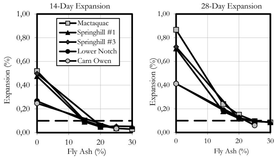
FIGURE 1: Accelerated mortar bar test results for Belldune (Type F) fly ash after a) 14 days and b) 28 days.
