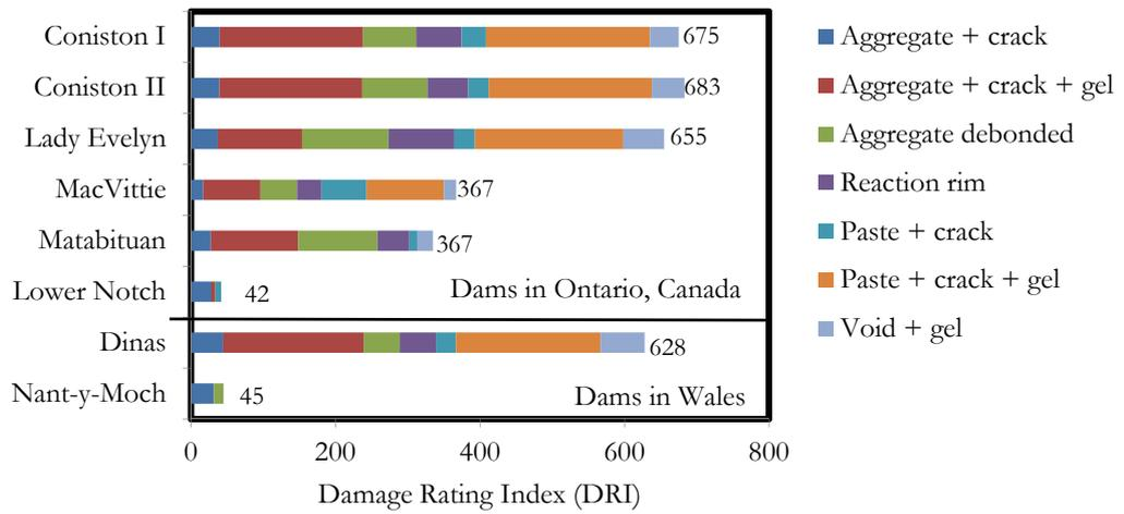
FIGURE 6: Damage Rating Index (DRI) of Dams in Ontario, Canada and Wales produced with and without Fly Ash (Thomas et al., 2012).
