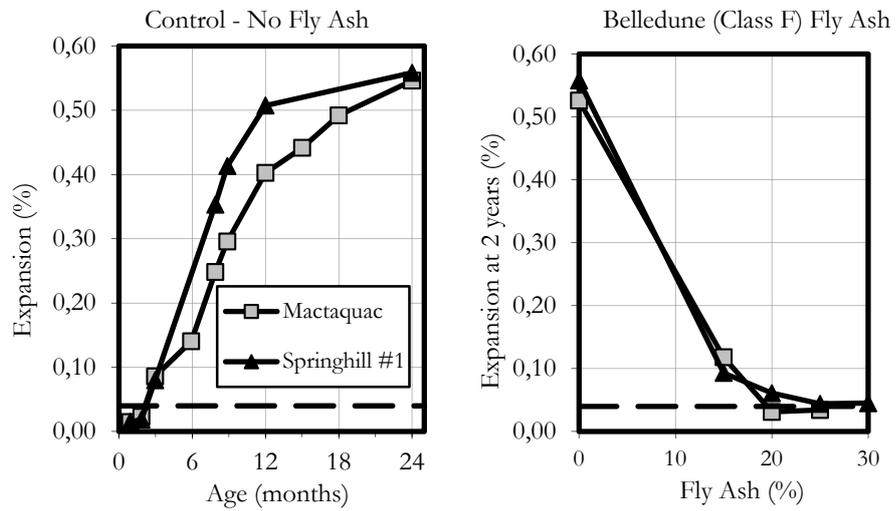
FIGURE 2: ASTM C1293 Concrete prism test results for Belldune (type F) fly ash for both Mactaquac and Springhill aggregate.
