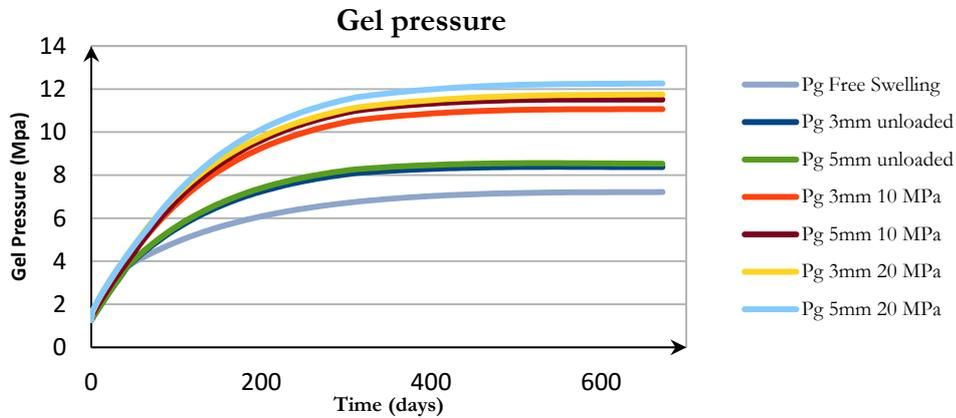
FIGURE 7: Gel pressure from the model in restrained tests.
