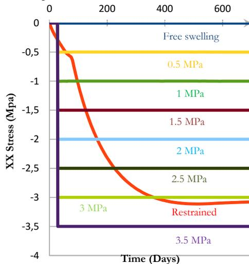
FIGURE 9: Stresses in direction XX (MPa).
