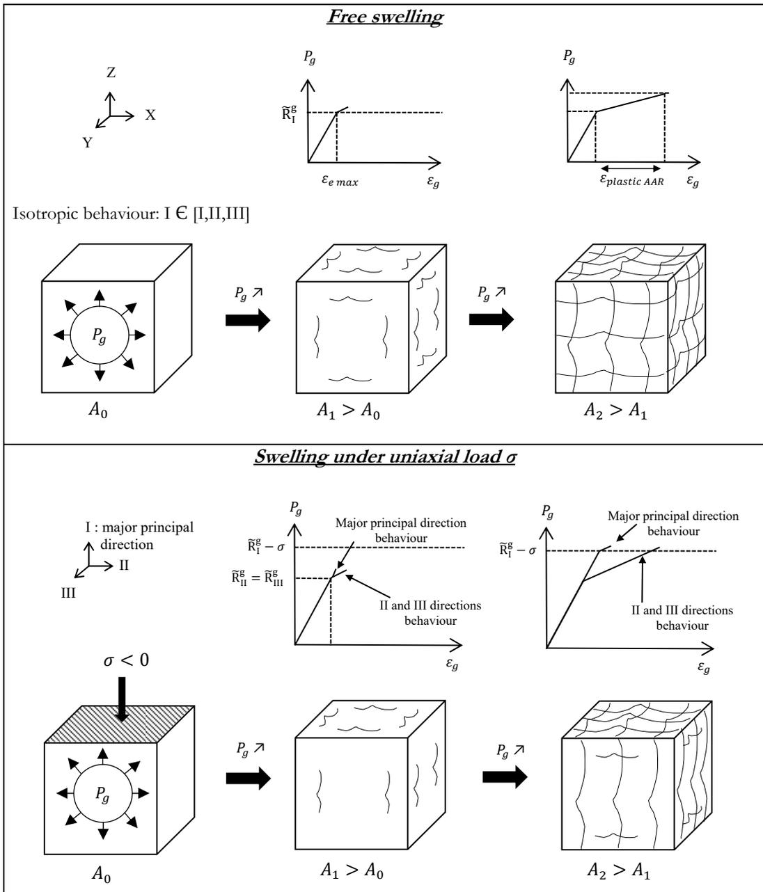
FIGURE 3: Loading effects on cracking direction on specimen affected by ASR.
