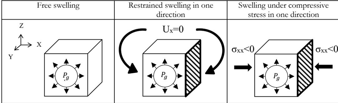
FIGURE 8: Conditions of theoretical tests.
