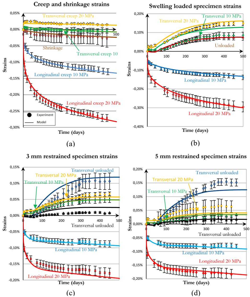
FIGURE 5: Multon's tests [1]: (a) creep and shrinkage without ASR, (b) ASR free swelling tests, (c) 3 mm restrained tests, (d) 5 mm restrained tests ( $R_t=3.7$  MPa;  $\phi_g^\infty=0.0078$  m<sup>3</sup>/m<sup>3</sup>;  $\phi_g^v=0.00148$  m<sup>3</sup>/m<sup>3</sup> bg=0.25;  $M_g=27700$  MPa;  $H_{asr}=0.1$ ).
