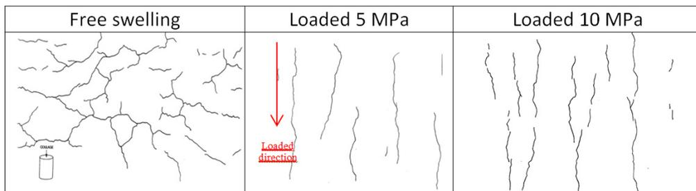
FIGURE 4: ASR specimens cracking appearance due to several loadings [3].
