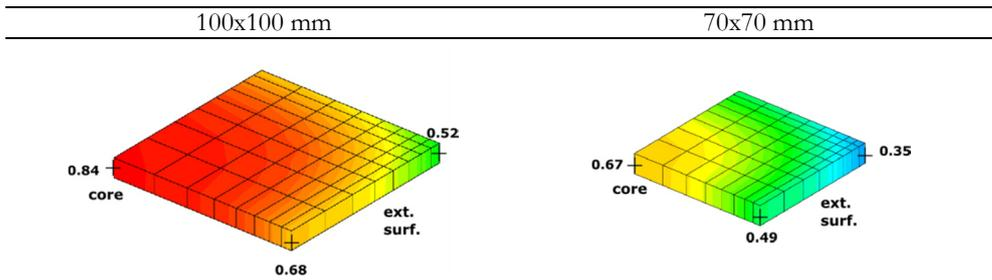
FIGURE 7: Advancement of ASR in one size of aggregate in the specimens of Lindgard's experiments [3] after 100 weeks.
