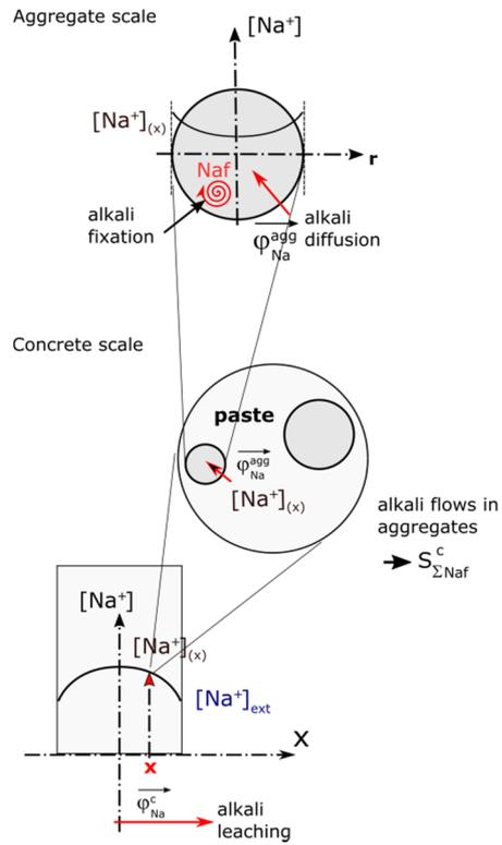
FIGURE 1: Alkali mass balance at aggregate and at concrete scale.
