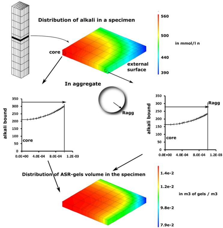
FIGURE 5: 100x100 mm cross section subjected to ASR in leaching condition. Top: distribution of alkali in specimen, middle: gradient of bound alkali in aggregates in the core and at the external surface of the specimen, bottom: resulting distribution of ASR-gels in specimen.
