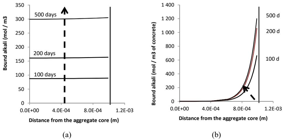
FIGURE 4: Alkali bound in ASR-gels for an aggregate of mean diameter of 2 mm: (a) aggregate with slow reactivity, (b) aggregate with high reactivity.
