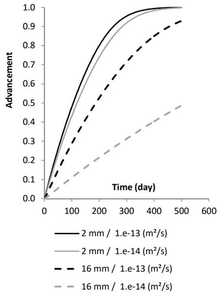
FIGURE 3: Kinetics of gel formation for two coefficients of diffusion and the same characteristic time of reaction for two sizes of aggregate (mean diameters 2 and 16 mm).
