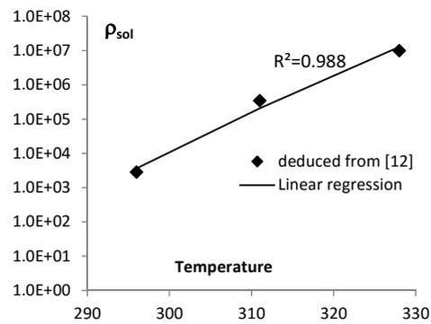
FIGURE 2: Determination of alkali threshold with temperature.
