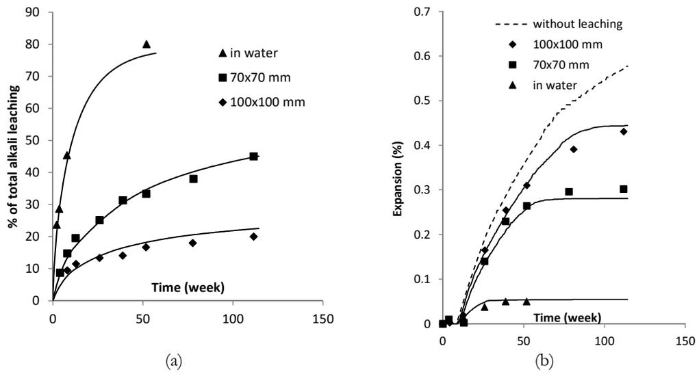
FIGURE 6: Alkali leaching (a) and expansion (b) in Lindgard's experiments [3] (points) and numerical modelling (curves).
