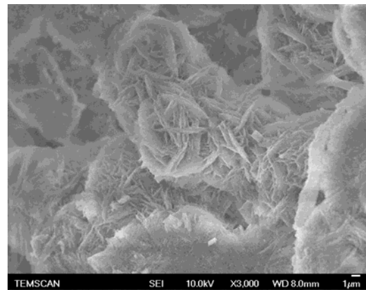
FIGURE 7: Photomicrographs of GP mortar at 170 days. ASR product with a "rosette-type" morphology.
