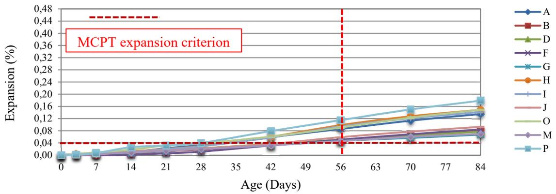
FIGURE 5: Expansion behavior of the moderately reactive fine aggregates (MCPT).
