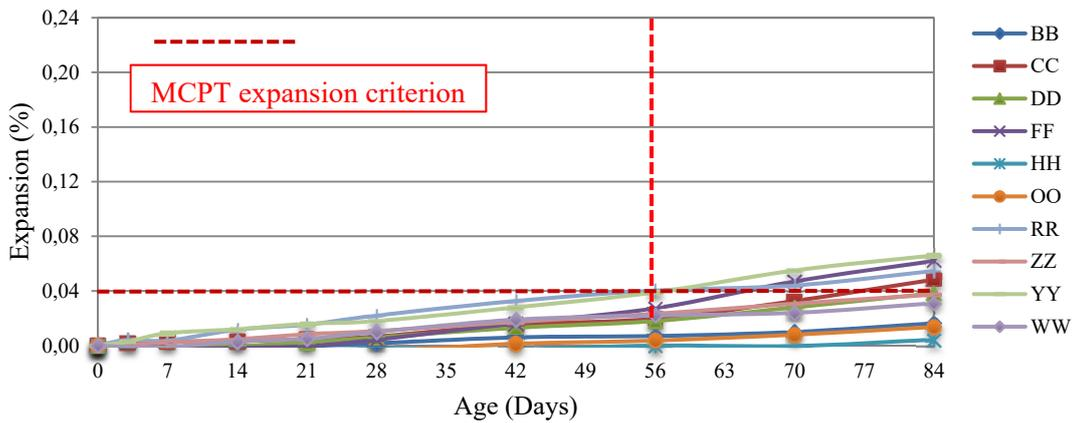
FIGURE 3: Expansion behavior of the slow/low reactive and non-reactive coarse aggregates (MCPT).
