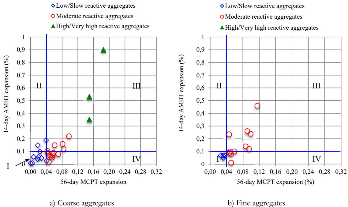
FIGURE 8: Correlation between AMBT and MCPT results: a) Coarse aggregates; b) Fine aggregates.
