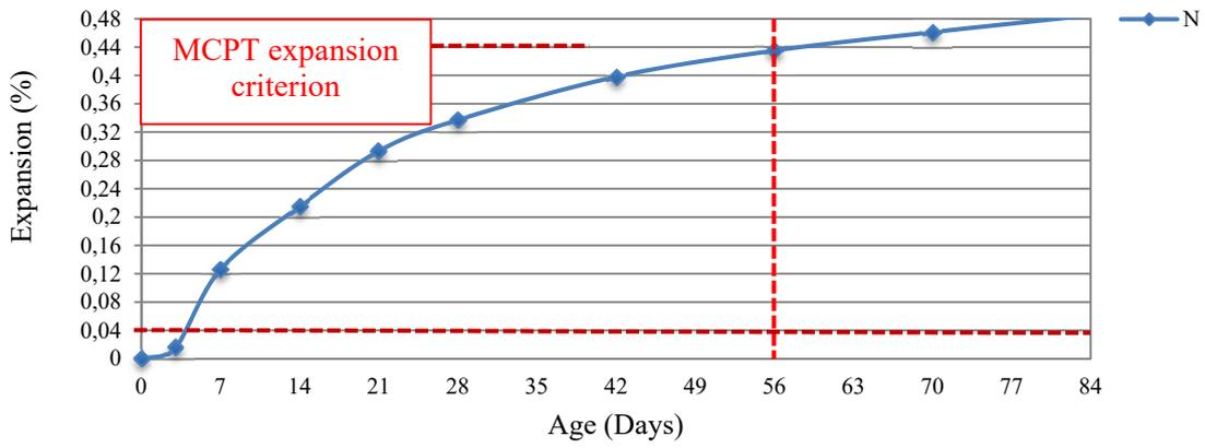
FIGURE 4: Expansion behavior of the high/very highly reactive fine aggregates (MCPT).
