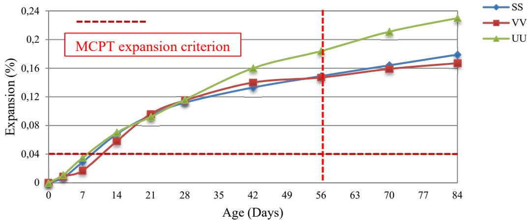
FIGURE 1: Expansion behavior of the high/very highly reactive coarse aggregates (MCPT).
