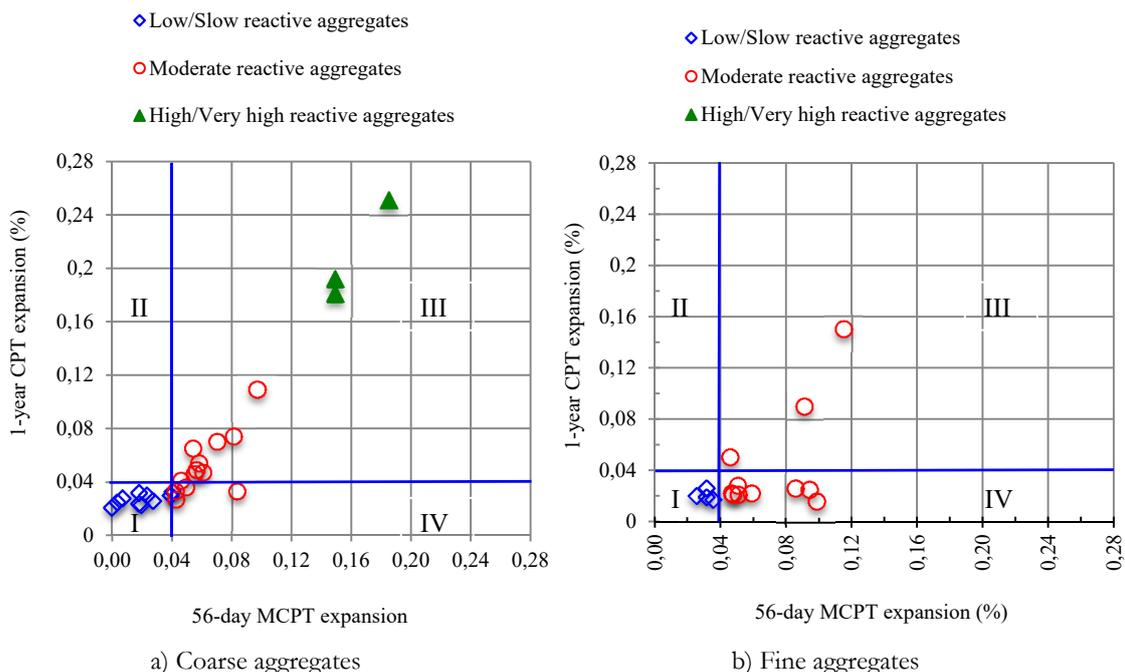
FIGURE 7: Correlation between CPT and MCPT results: a) Coarse aggregates; b) Fine aggregates.
