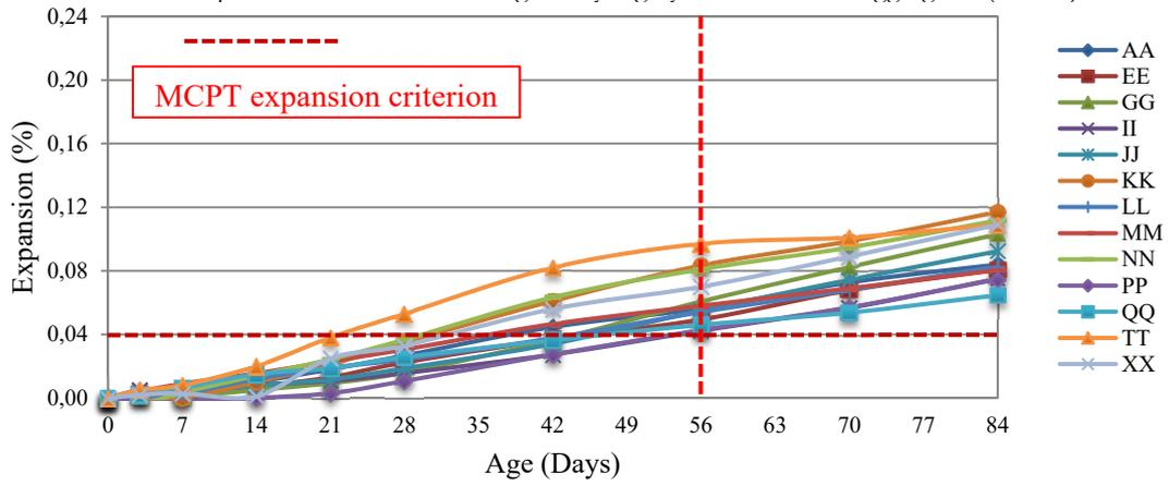
FIGURE 2: Expansion behavior of the moderately reactive coarse aggregates (MCPT).
