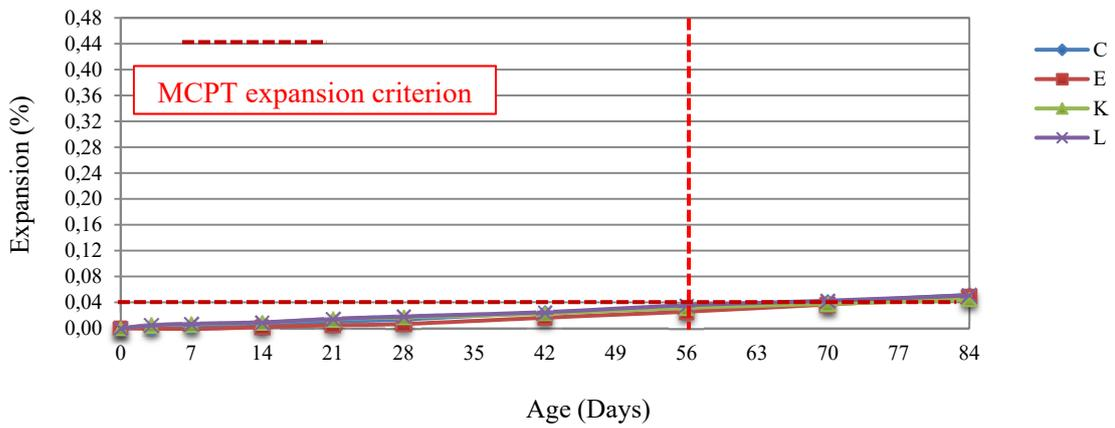
FIGURE 6: Expansion behavior of the non-reactive fine aggregates (MCPT).
