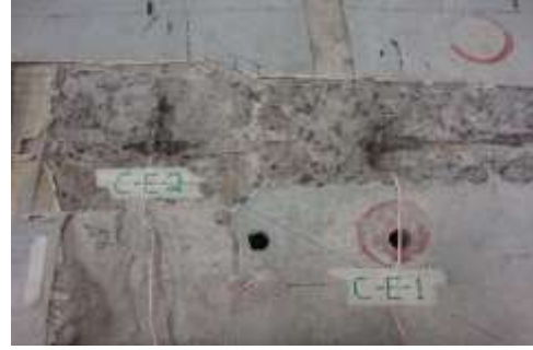
FIGURE 2: RBC columns pictures: A) concrete cover removal and preparation of the surface underneath the stirrups; B) Stirrups with strain gauges glued for measurements of stress-relief white cutting.
