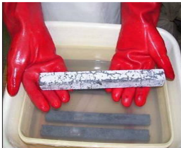
FIGURE 4: Cracking in mortar bar.
