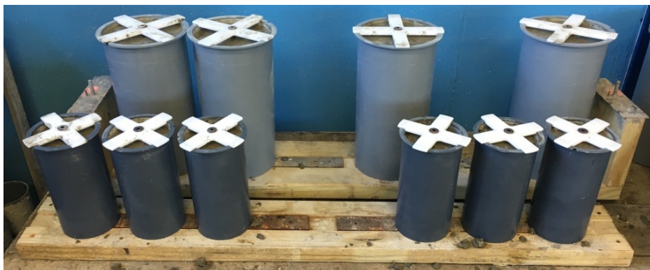
FIGURE 5: Photo of CCT specimens in the "Stace-molds" apparatus (105x305 mm in back and 100x200 mm in the front).
