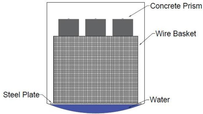
FIGURE 2: Schematic of the autoclave interior with concrete prisms inside.
