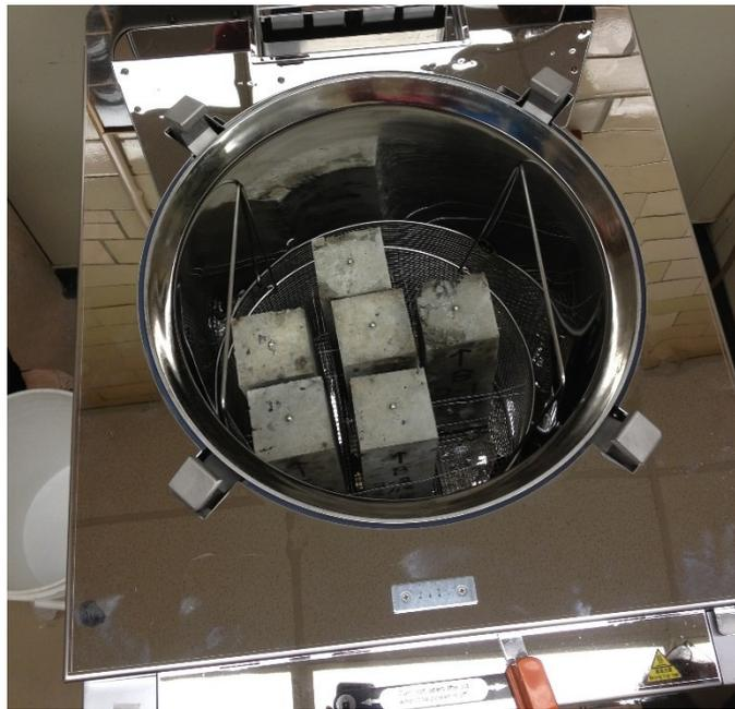
FIGURE 1: Concrete prisms standing upright inside the autoclave.
