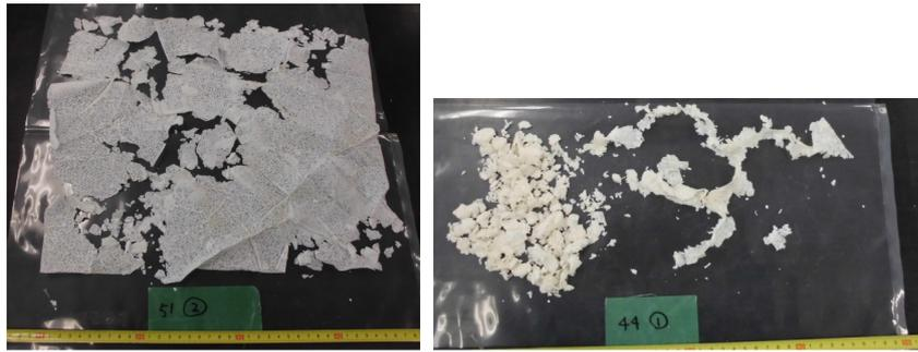
(a) Aggregate T, alkali = 3.00 kg/m<sup>3</sup>, 60 °C (b) Aggregate N, alkali = 2.00 kg/m<sup>3</sup>, 60 °C.
