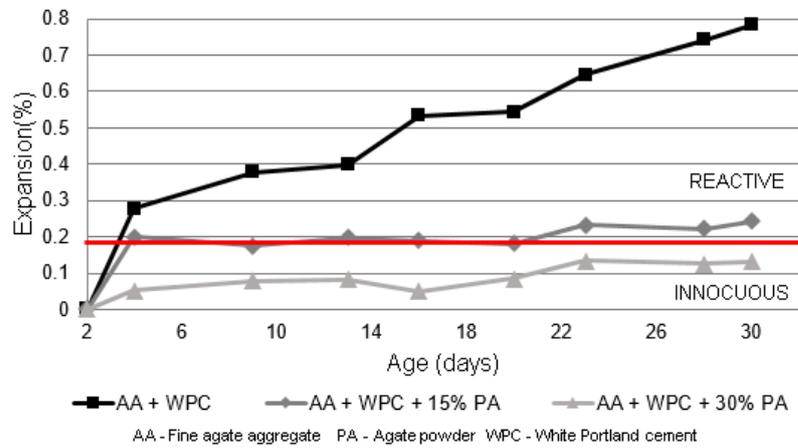
FIGURE 6: Expansions measurements of the samples produced with white Portland cement.
