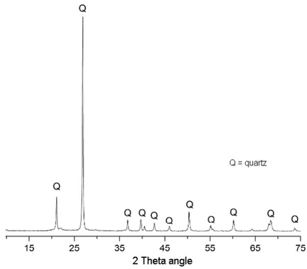
FIGURE 2: X ray diffractometer of the fine agate aggregate.
