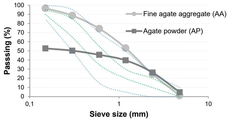
FIGURE 3: Particle size distribution of the fine agate aggregate and agate powder.
