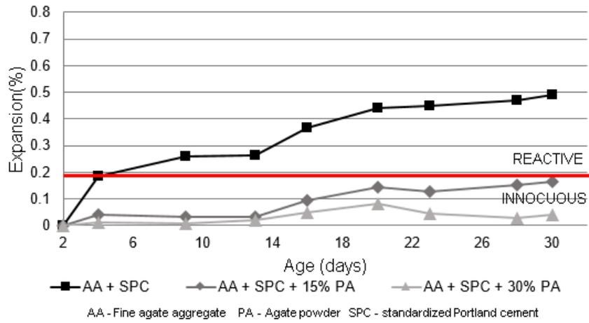
FIGURE 5: Expansions measurements of the samples produced with standardized Portland cement from SPC.
