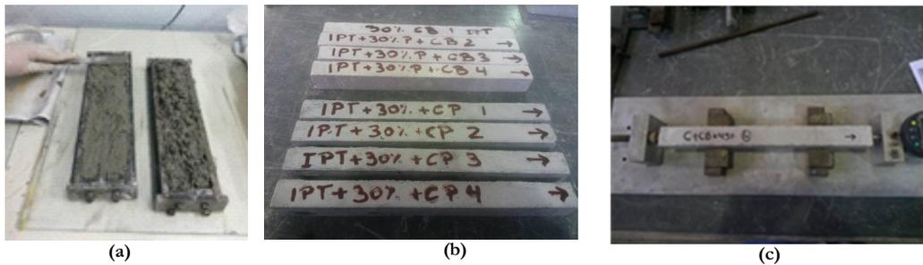
FIGURE 4: Alkali silica reaction test. A) Samples production; B) Samples produced; C) Measurements with the extensometer.
