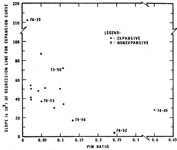
Fig. 10 Plot showing relation between the ratio of porosity to microcrystalline content (P/M ratio) of aggregates and expansivity of concrete made with those aggregates and high alkali cement.
