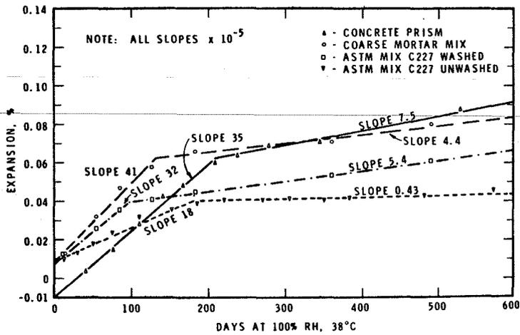
Fig. 6 Effect of variation in grain size of aggregates on expansion of concrete prisms and mortar bars made with high alkali cement. Slopes of the regression lines of the expansion curves vary from  $18 \times 10^{-5}$  to  $55 \times 10^{-5}$  with increasing grain size of aggregate.
