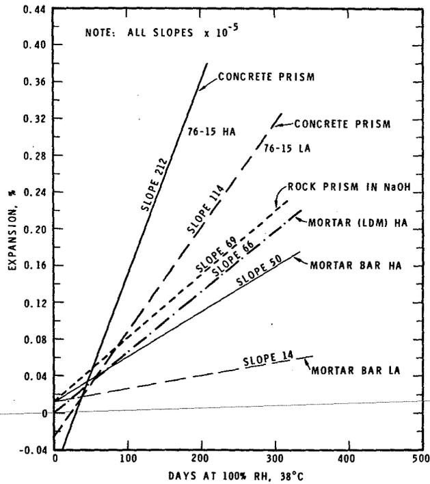
Fig. 7 Expansions of concrete prisms and mortar bars made with argillite 76-15 and high and low alkali cements. (The slope of expansion curve for rock prisms in NaOH is also shown; for comparison, the slope of expansion of mortar bars made with cement containing 0.96 per cent  $\text{Na}_2\text{O}$  equivalent by Dolar-Mantuani (5) is also shown, line LDM.)
