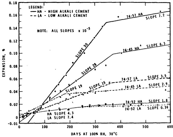
Fig. 3 Graph showing expansions of some typical concrete prisms made with expansive and nonexpansive aggregates and high and low alkali cements. Each point on the graph represents the average expansion of a pair of prisms
