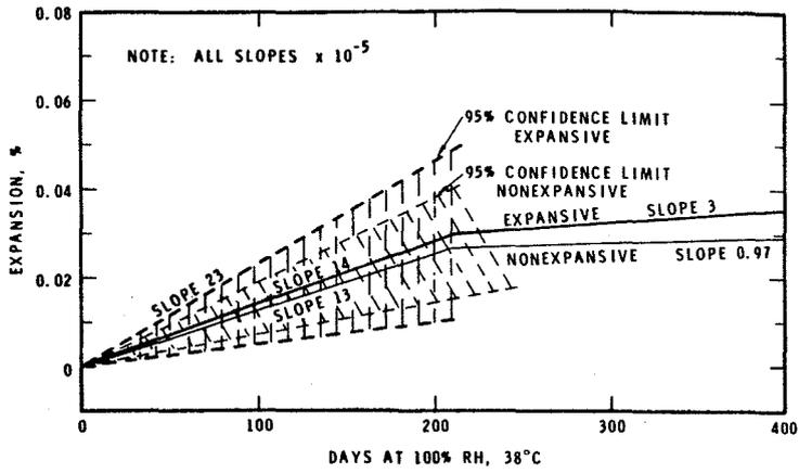
Fig. 5 Regression lines representing mean expansion of all concrete prisms made with low alkali cement
