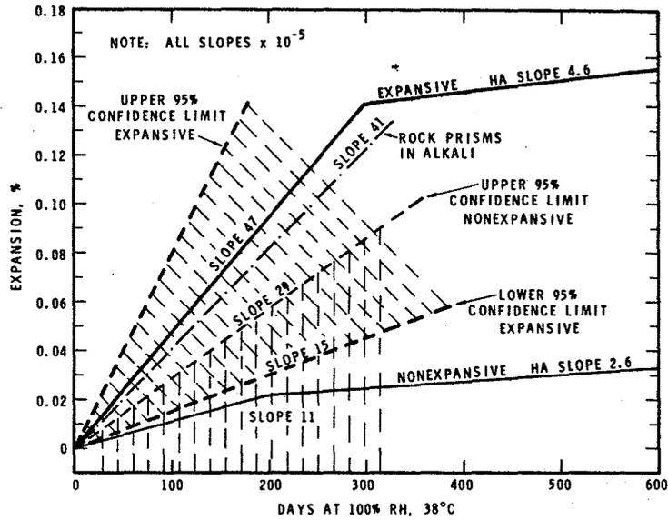
Fig. 4 Regression lines for early and late stages of expansion of the means of all curves for concrete prisms made with high alkali cement. (Separate lines are shown for expansive and nonexpansive aggregates; for purposes of comparison, the slope of the regression line for the expansion of the mean of all rock prisms in alkali is also shown.)
