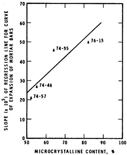
Fig. 8 Graph showing relation between content of microcrystalline material in expansive argillites and quartzwackes and expansion of mortar bars made with them and high alkali cement. The expansivity of the samples is shown by the slope of the regression line of the expansion curve
