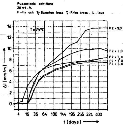
Fig. 5 Influence of puzzolanic additions on the expansion of mortar bars
