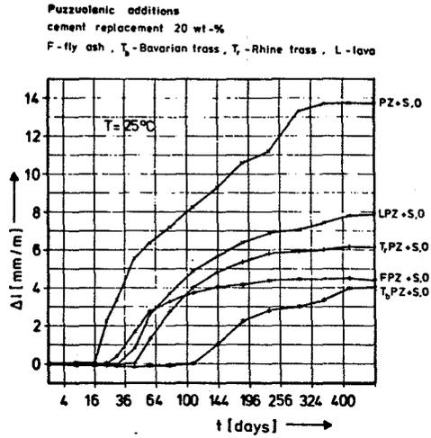
Fig. 7 Expansions of mortars containing the puzzuolanas as cement replacement
