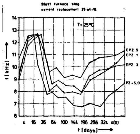
**Fig. 9** Natural frequencies of the mortar bars containing blast furnace slag
