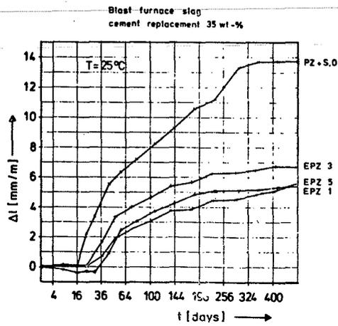
Fig. 8 Expansions of the mortar bars containing blast furnace slag
