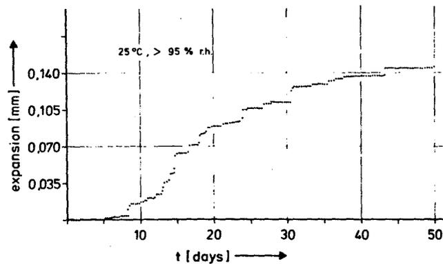
Fig. 10 Quasi-continuous expansion measurement
