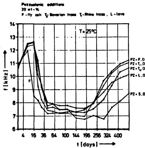
Fig. 6 Natural frequencies of the mortar bars containing puzzolanas
