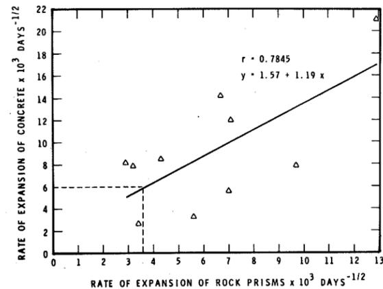
FIGURE 6: Correlation between expansion of miniature rock prisms in 2 N NaOH and concrete prisms made with high alkali cement made with Sudbury aggregates. The correlation coefficient is 0,7845.
