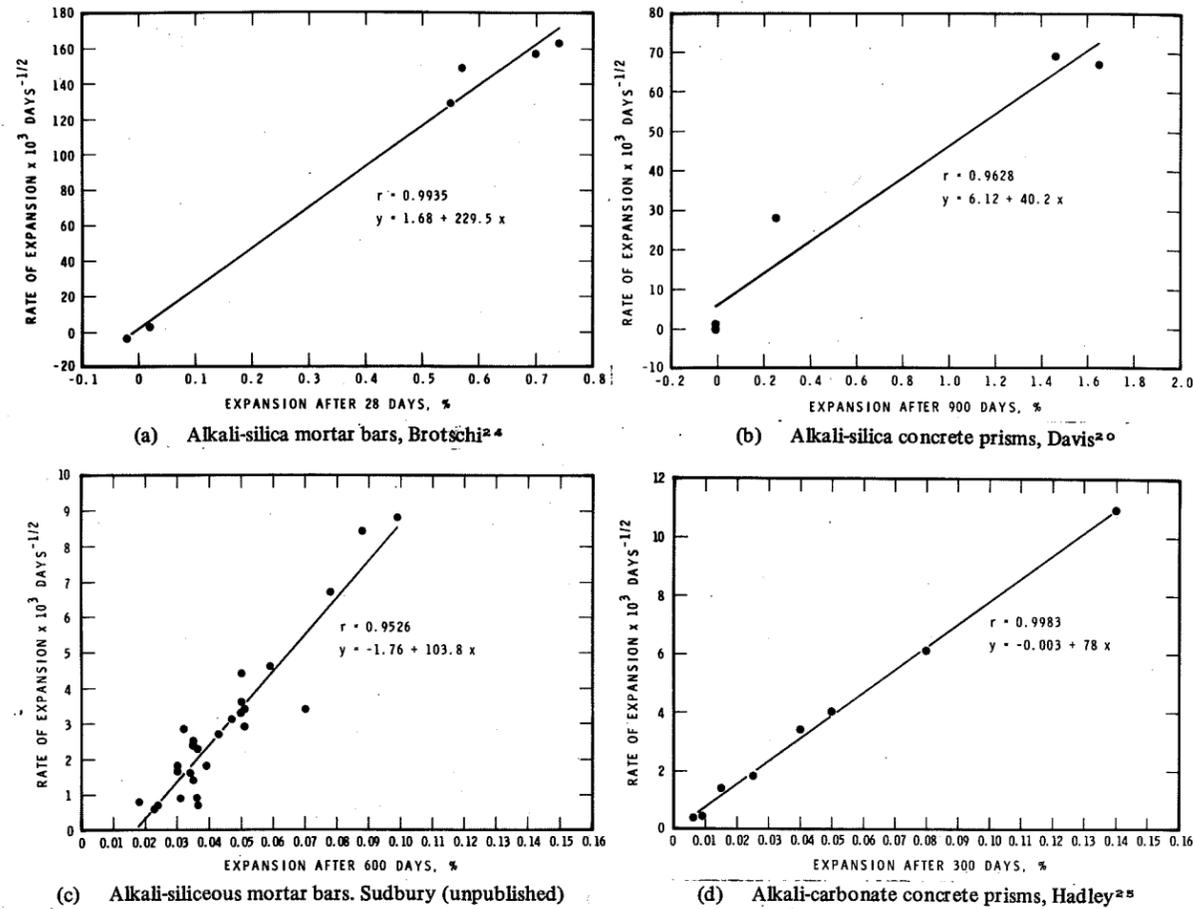
FIGURE 3 : Percentage expansions after varying times vs rates of expansion of mortar bars and concrete prisms showing the correlation between rate of expansion and the final expansion of the samples. Also included are the correlation coefficient  $r$  and the equation for each line fitted to the points in the graphs.
