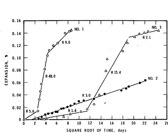
FIGURE 4: Characteristic expansions of concrete prisms made with alkali-silica reactive aggregate No 1, alkali-carbonate expansive aggregate No 2 and slowly expanding siliceous aggregate No 3. The rates of expansion 'R' x 10<sup>3</sup> are indicated for the three phases of the expansions.
