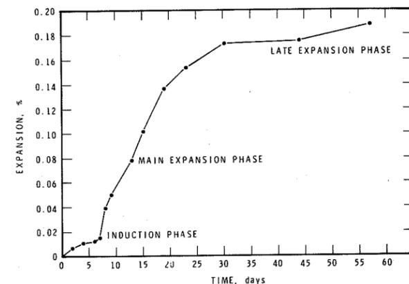
FIGURE 1: Typical expansion curve of mortar bars made with sand containing opal.
