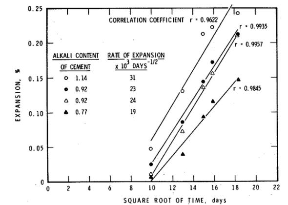
FIGURE 2: Linear relationship between the percentage expansion of mortar bars made with reactive sand and cements with varying alkali contents (after Stanton<sup>19</sup>).
