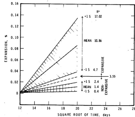
FIGURE 5: One standard deviation (s) time-expansion envelopes about the mean expansion, of expansive and non-expansive concrete prisms. The cut-off rate,  $3.55 \times 10^{-3} \text{ days}^{-1/2}$ , used to differentiate between expansive and non-expansive concrete prisms is also shown. \* R is the rate of expansion expressed as  $\text{days}^{-1/2} \times 10^3$ .
