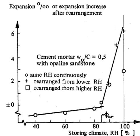
FIGURE 4: Effect of atmospheric humidity on expansion due to the alkali-silica reaction; data from Lenzner & Ludwig<sup>5</sup>.
