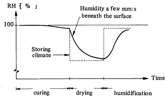
FIGURE 5: Approximate 'moisture history' for reactive grains close to the surface and the storing climate of the specimens
