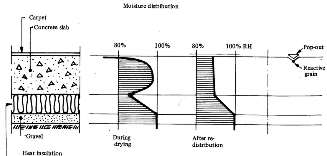
FIGURE 1 : Typical floor structure and moisture distribution of a concrete slab laid directly in the ground
