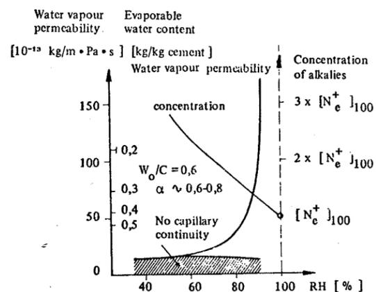
FIGURE 2 : Examples of the influence of moisture on some factors participating in the alkali-silica reaction. Data from Nilsson (1980).
