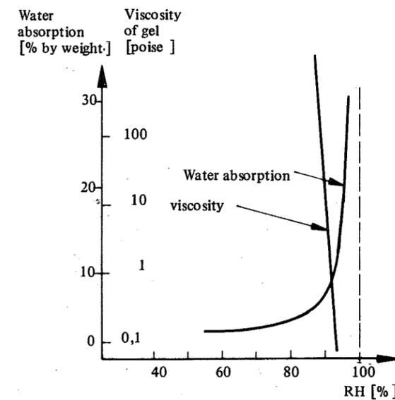
FIGURE 3: Examples of the influence of moisture conditions on the behaviour of an alkali-silica gel; absorption data from Krogh<sup>3</sup> and approximate viscosity data from Moore<sup>4</sup>.
