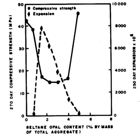
Influence of reactive aggregate content upon compressive strength and expansion. w/c 0,59, a/c 4,5, reactive particle size 150 to 300  $\mu\text{m}$ . Acid soluble alkali content of the cement, ( $\text{Na}_2\text{O}$ ) = 1,04%
