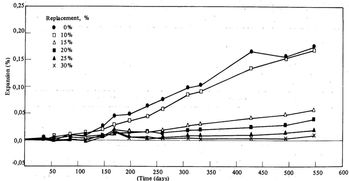
FIGURE 5 : Influence of different amounts of calcined shale replacing cement on linear expansion of concrete prisms stored over water in sealed containers at 38 °C, cement H = 0,97% Na<sub>2</sub>O eq and 350 kg/m<sup>3</sup>; aggregate = hornfels P5<sub>3</sub>.
