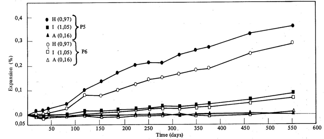
FIGURE 1 : Linear expansion of mortar prisms made with aggregates P<sub>5</sub> and P<sub>6</sub> and each of the cements H(0,97), I(1,05) and A(0,16). Stored over water in sealed containers at 38 °C; a/c ratio 1,5
