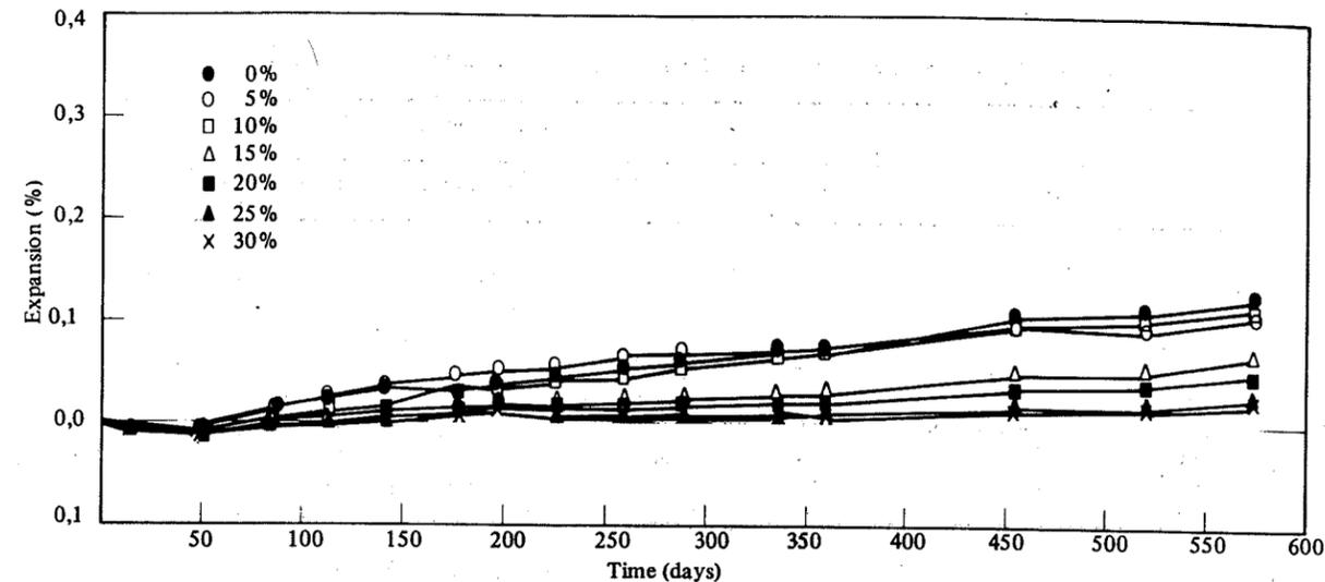
FIGURE 4 : Influence of different amounts of calcined shale (JCS) replacing high alkali cement H(0,97) on the linear expansion of mortar prisms stored over water in sealed containers at 38 °C. Aggregate, hornfels P5<sub>3</sub>, a/c ratio 2,25
