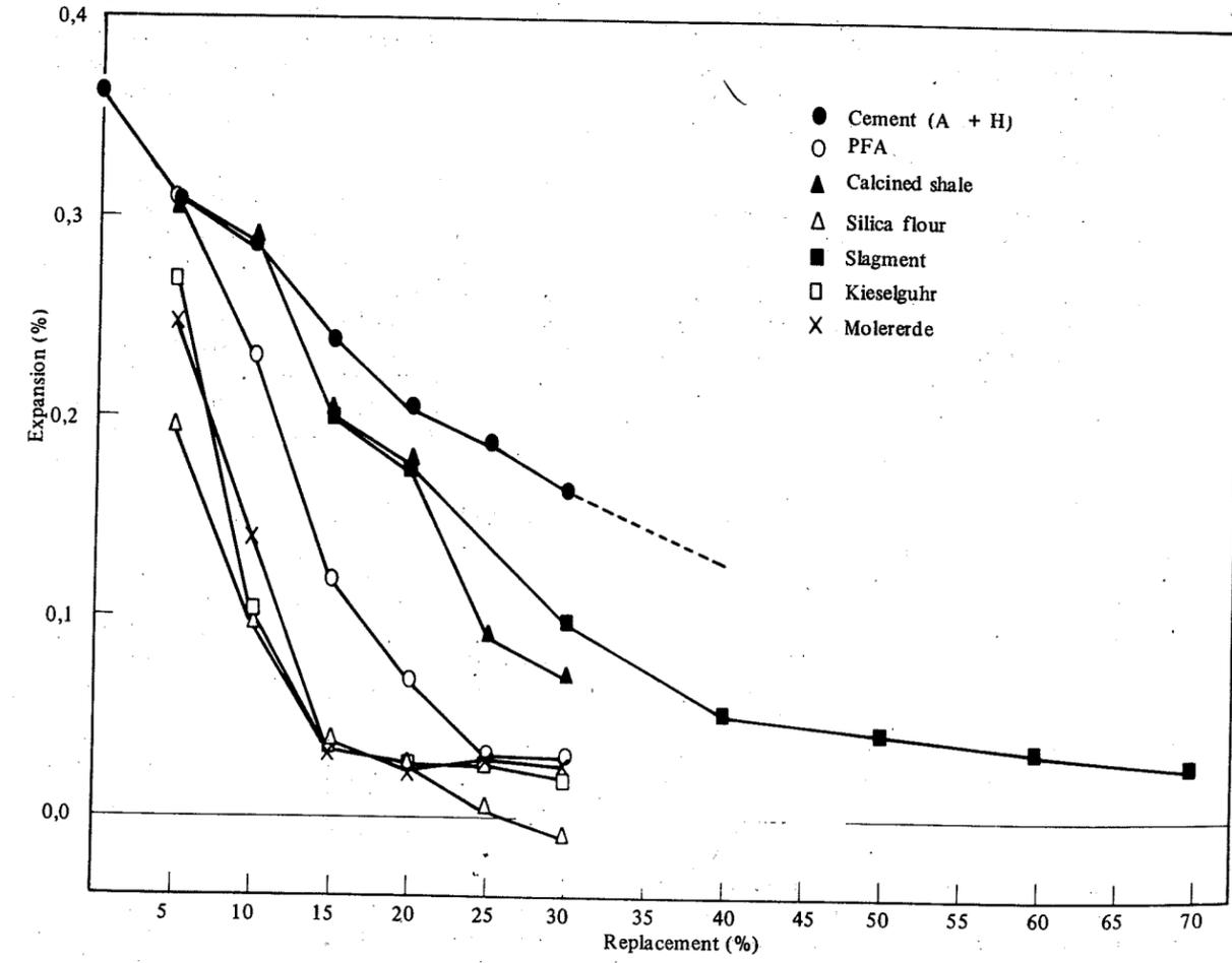
FIGURE 3 : Effect of replacing cement H(0,97) with increasing amounts of cement A(0,16) or various mineral admixtures, on the linear expansion of mortar prisms stored over water in sealed containers at 38 °C for 555 days. Aggregate, hornfels P<sub>5</sub>; a/c ratio 1,5.
