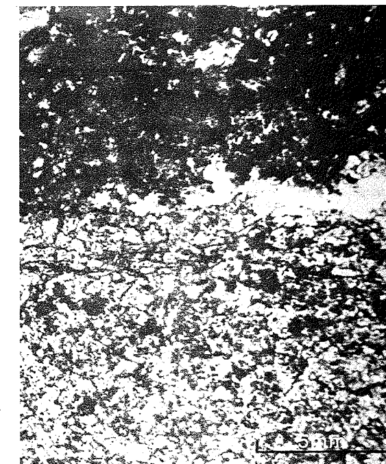
FIGURE 4: A petrographic thin section micrograph showing microcracks developed in the rim zone.
