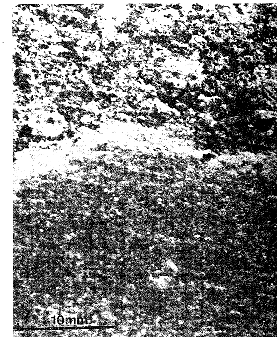
FIGURE 3: The development of a white rim at the margin of a dolomitic limestone aggregate particle.
