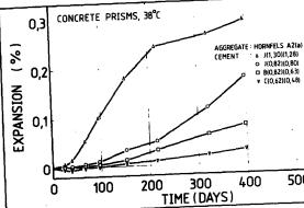
'acid soluble alkali content'. The first figure in brackets after a cement number, he explained, referred to the acid soluble alkali content and the second figure to the available alkali content, expressed as per cent Na<sub>2</sub>O equivalent. It could be seen that cements J(0,82)(0,80) and B(0,82)(0,63) had the same acid soluble alkali content but different available alkali contents. Cement J with the higher available alkali content had given the higher expansion.
