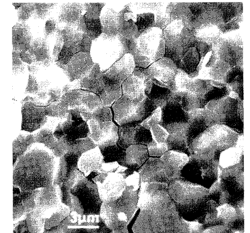
Fig. 14. Microcrystalline and microcracked dolomitic aggregate.
