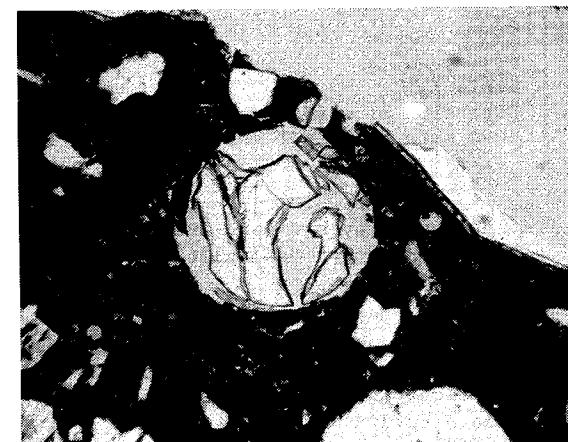
Fig. 5. Thin-section showing alkali-silica gel in an air void in the cement paste. Magnification 60x. Transmitted light.
