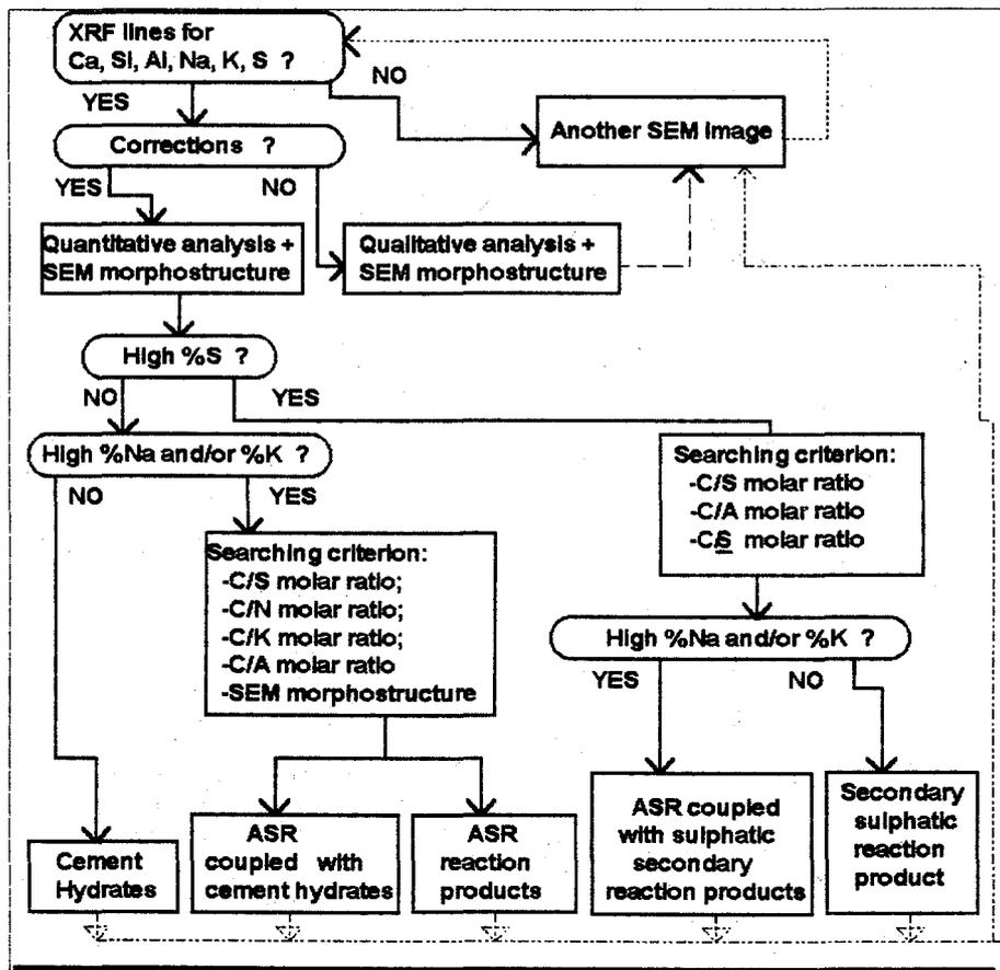
Figure 2. Flow chart for the ASR diagnosis by electron microanalysis
