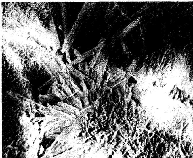
*Figure 3. SEM image for the cement paste morphostructure damaged by ASR products associated with secondary sulphate reaction products.*
