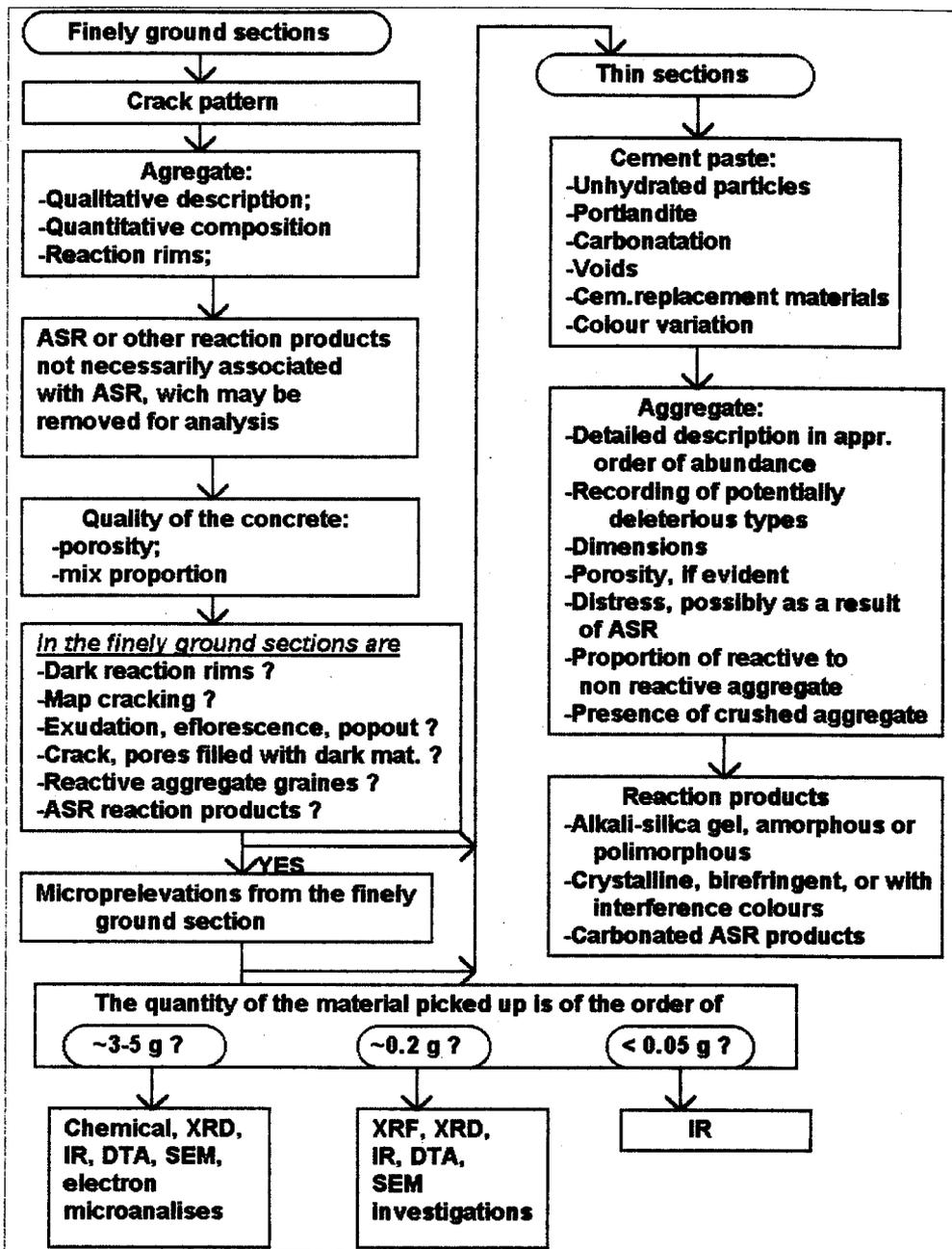
Figure 1. Flow chart for the concrete diagnosis and/or investigation of ASR by optical microscopy and connections with other analysis.
