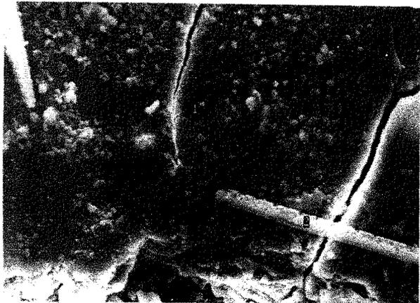
**Figure 2.** Reactive carbonate aggregate grain, (7), with botroydals reactions products, (8), (9), (10), on the corroded surface. The phenomena of cracking appear between the compact and amorphous AAR gel, (1), (2), (3), (6), and the hardened cement paste, (4), (5).
