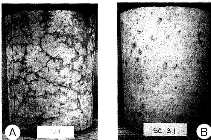
Fig. 3 Unsealed (A) and silane-sealed (B) concrete cylinders exposed to cycle C4, after 1.5 years.
