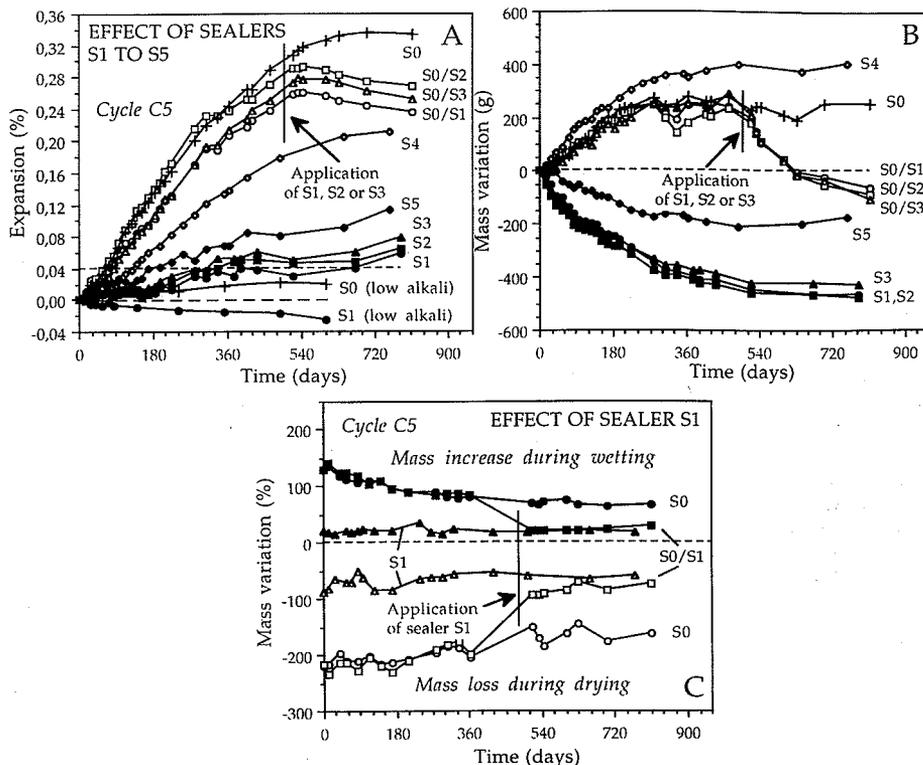
Fig. 4 Expansion (A), cumulative mass variation (B) and mass variation during drying and wetting (C), for sealed and unsealed concrete cylinders exposed to cycle C5.
