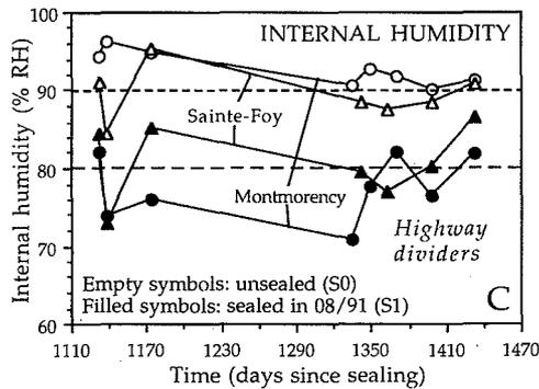
Fig. 5 Unsealed and silane-sealed (S1) sections of highway dividers in Montmorency (A) and in Sainte-Foy (B), and corresponding internal humidity during the last year (C).
