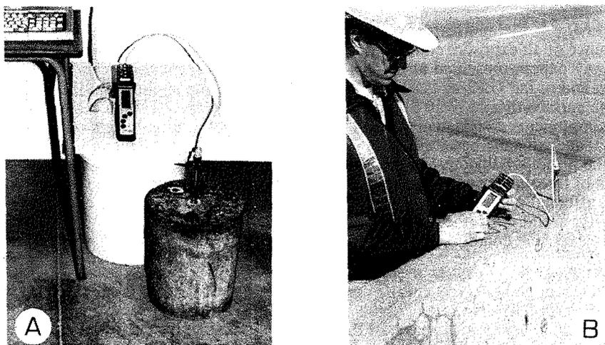
Fig. 1 Humidity measurements in concrete cylinders (A) and highway dividers (B).
