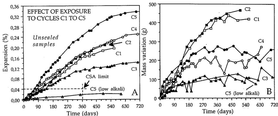
Fig. 2 Expansion (A) and mass variation (B) of unsealed concrete cylinders submitted to exposure cycles C1 to C5.
