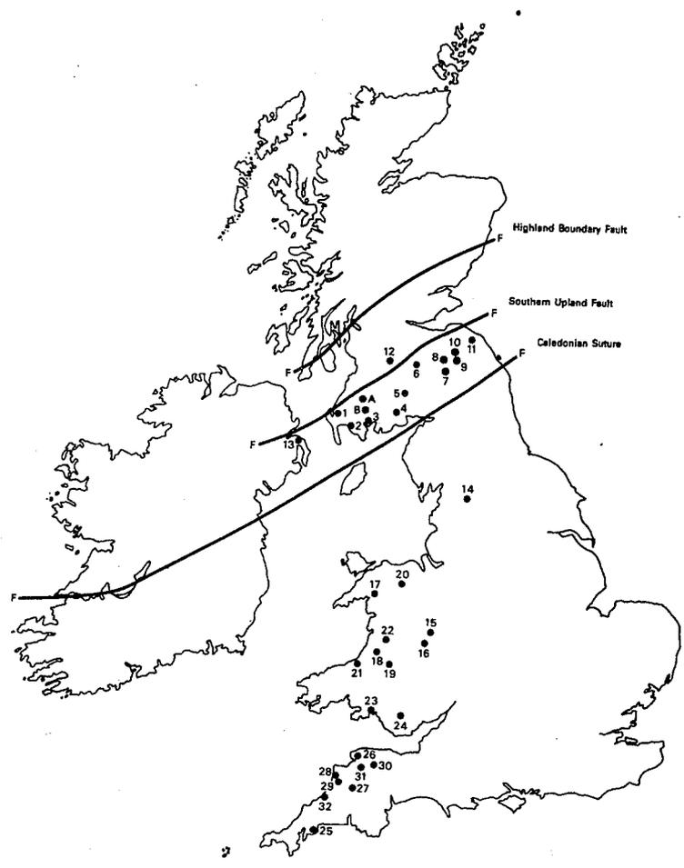
FIGURE 2: Regional survey of UK greywacke, showing sample collection locations (results of laboratory testing of these samples are shown in table 1.)
