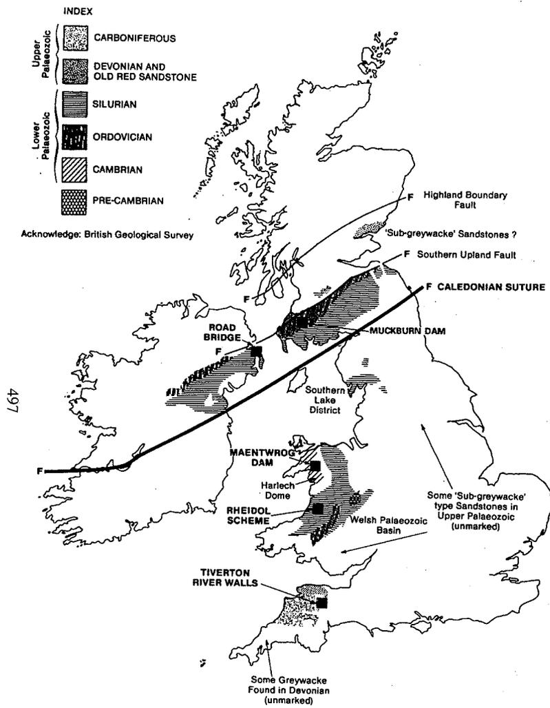
FIGURE 1: Geological map showing strata by geological age where greywacke are found in the UK. Also located are the greywacke containing structures which show distress due to AAR.
