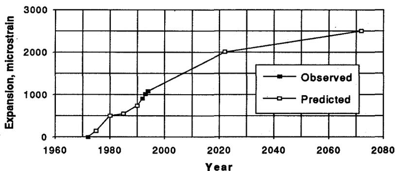
Fig. 3 Observed and predicted expansions for the Intake Tower
