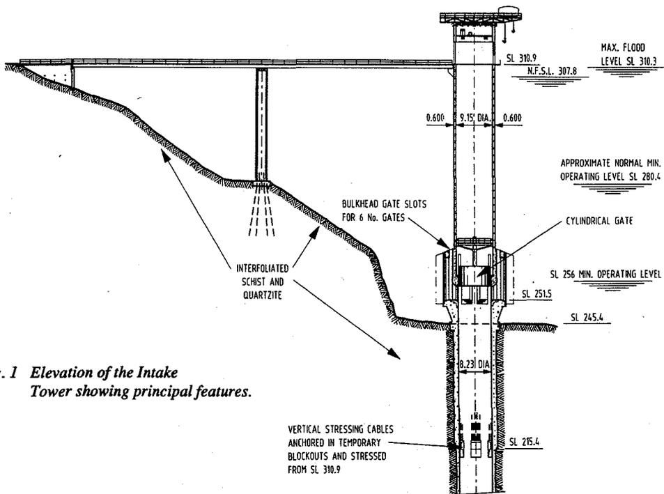
Fig. 1 Elevation of the Intake Tower showing principal features.
