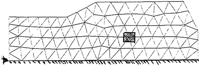
Fig 2 : Mesh used for numerical computation of concrete elements and boundary conditions
