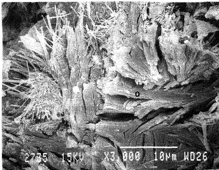
Fig 8 : Cement B, 2d at 20°C, 100d at 38°C, secondary ettringite (o)
