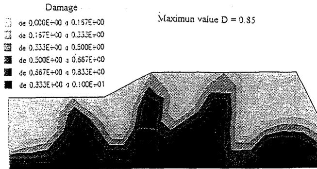
Fig 3 : Damage in concrete tie after three days
