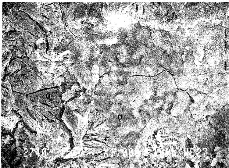
Fig 7 : Cement A, cycle I, 100d at 38°C. Coexistence of AAR gel (+) and secondary ettringite (o)
