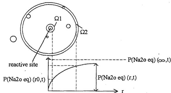
Fig 4 : Evolution of the probability of  $\text{Na}_2\text{O}_{eq}$  versus  $r$ , size of reactive silica particle
