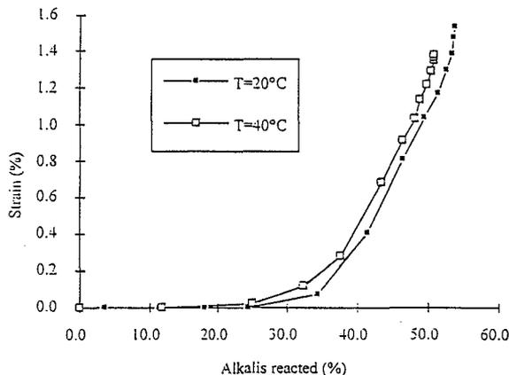
Fig 1 : Evolution of strain versus alkalis reacted
