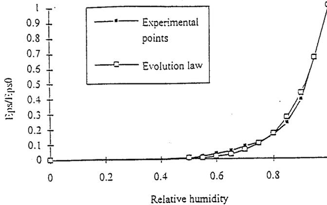
Fig 4 : Evolution of expansion versus relative humidity, comparison between experimental data and theoretical relation proposed.
