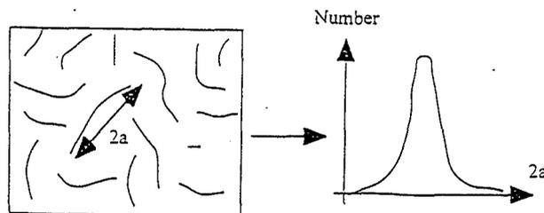
Fig 6 : Quantification of the initial cracking
