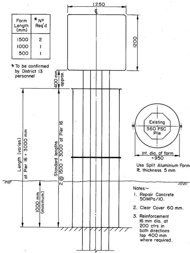
Fig. 3 Proposed repair technique
