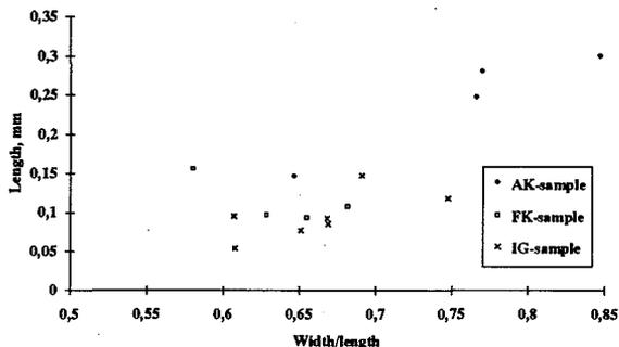
Figure 3. Morphology of SF in cement samples
