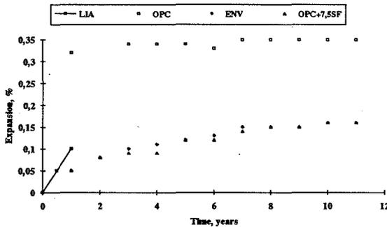
Figure 6. Measured expansion of various types of Portland cements, see the text for discussions. The solid line represents the limits set by Icelandic authorities (LIA).
