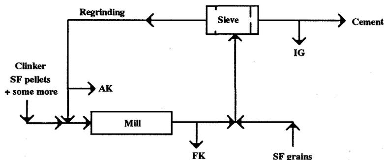
Figure 2. Schematics of the grinding process and location of sample sites and sample numbers.
