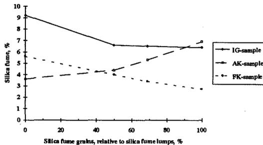
Figure 4. Calculated amount of SF in cement samples
