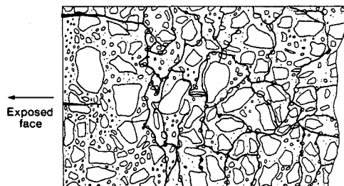
Fig. 1 Internal crack pattern which can be caused by ASR: reactive silica content in the coarser end of the sand fraction.
