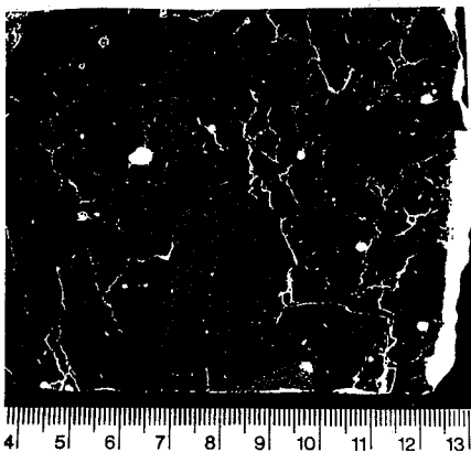
Fig. 3 Crack distribution in section taken from below rock fill level.
