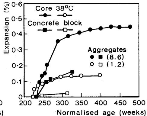
Fig. 10 Expansion predicted from core testing and actual expansion. 5.2 kg/m<sup>3</sup>.
