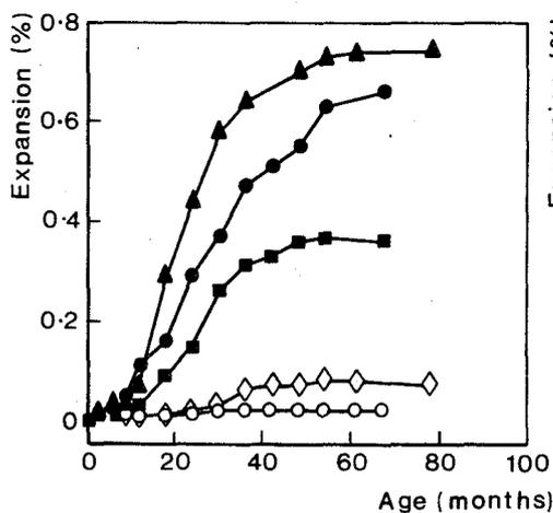
Fig. 1 Relationship between expansion and age.  $20^\circ\text{C}$ . Aggregate (3,6).
