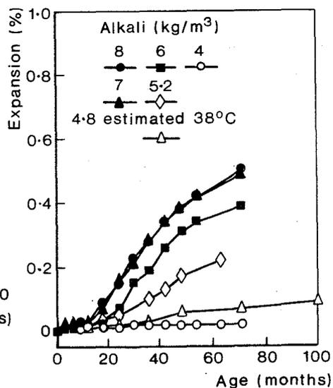
Fig. 2 Relationship between expansion and age.  $20^\circ\text{C}$ . Aggregate (8, 6).
