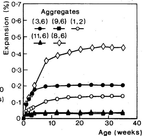
Fig. 8 Comparison of core expansions. 38°C. 5.2 kg/m<sup>3</sup>.
