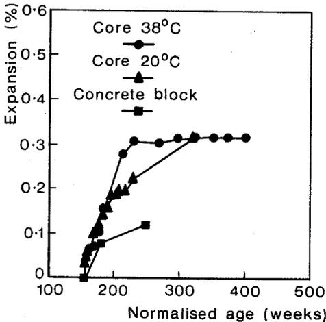
Fig. 9 Expansion predicted from core testing and actual expansion. Aggregate (11, 6). 7 kg/m<sup>3</sup>.
