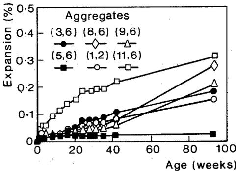
Fig. 7 Comparison of core expansions. 20°C. 7 kg/m<sup>3</sup>.
