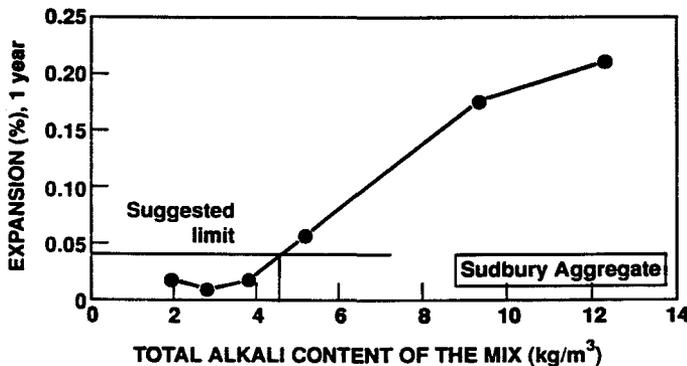
Fig. 4. Concrete prism expansions as a function of alkali loading for slowly reactive Sudbury aggregate (Rogers 1988).
