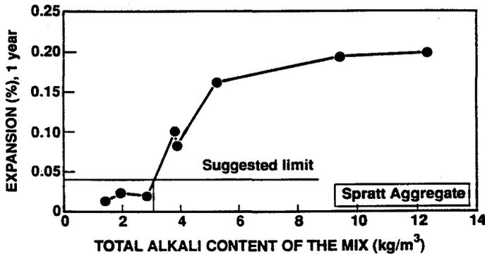
Fig. 3. Concrete prism expansions as a function of alkali loading for reactive Spratt aggregate (Rogers 1988).
