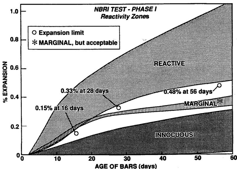
Fig. 2. Range of NBRI mortar bar expansions for aggregates with known field performance (Hooton, 1991).
