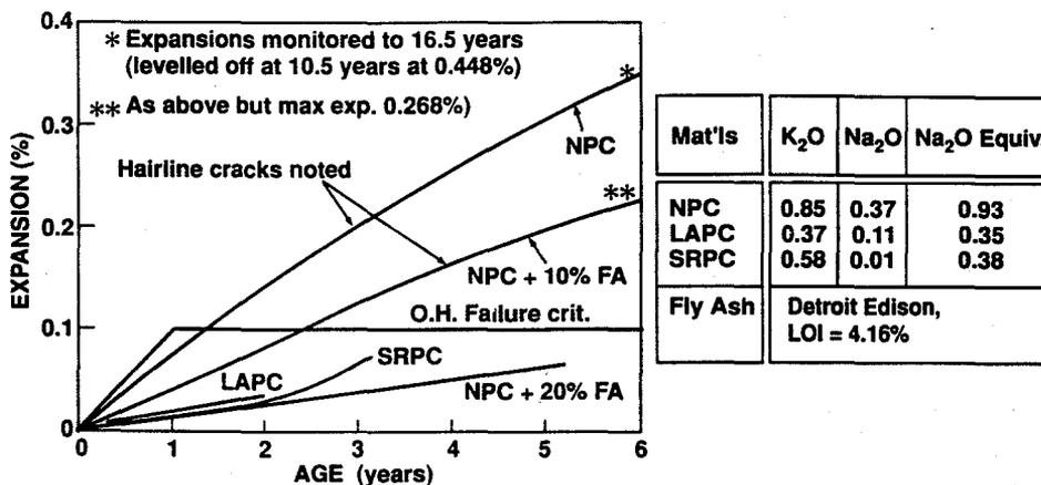
Fig. 1. ASTM C227 mortar bar expansions-greywacke with argillites crushed rock-Lower Notch GS - Effects of cement and fly ash.
