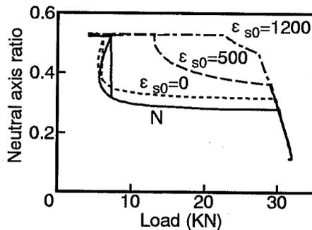
Fig. 7. Neutral axis ratio vs. load (analysis).
