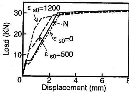
Fig. 6. Load-displacement diagram (analysis).
