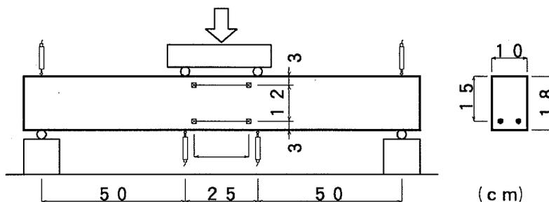
Fig. 1. Loading and measuring manner and cross section of beam.
