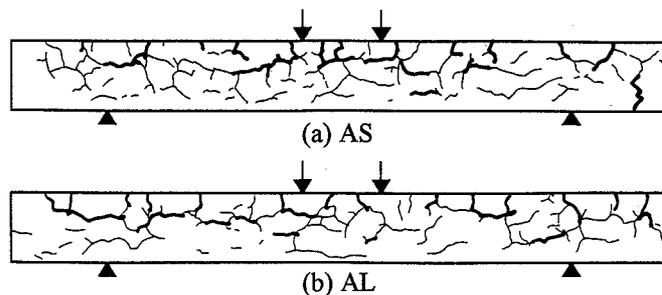
Fig. 2. Typical crack pattern of deteriorated beams
