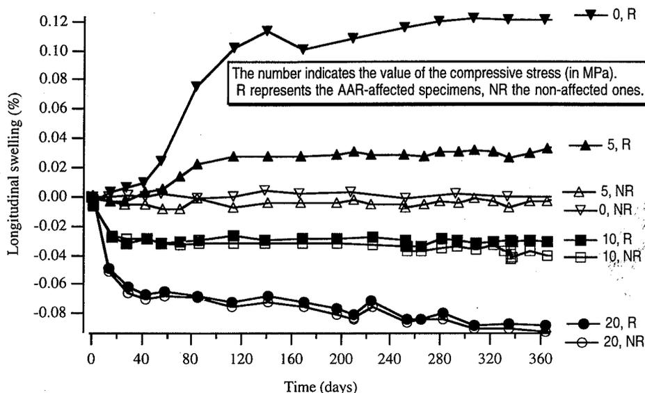
Fig. 4: Longitudinal swelling of specimens under uniaxial stress
