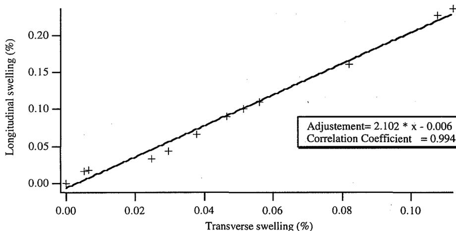
Fig. 6: Ratio between the longitudinal and transverse swellings
