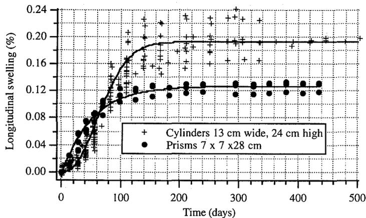
Fig. 2: Swelling of prisms and cylinders of the same composition, kept at 38°C, 100% R.H.
