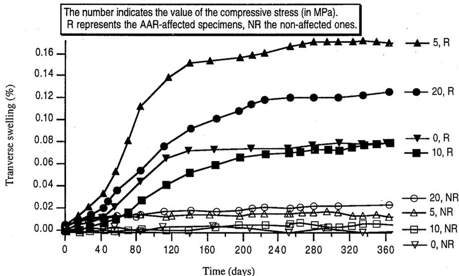
Fig. 5: Transverse swelling of specimens under a uniaxial stress
