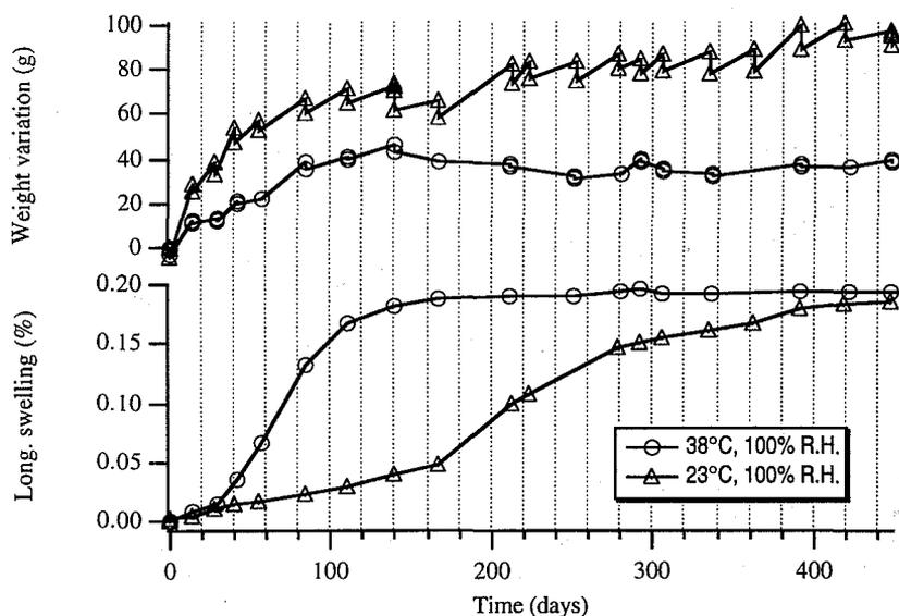
Fig. 3: Weight variation (upper) and longitudinal swelling (bottom) at 23 and 38°C
