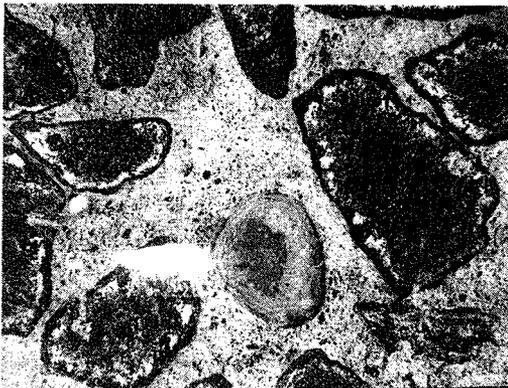
**Figure 3.** View of a fracture surface of a core showing reacted aggregate particles with dark outer rims and white inner rims. The matrix is impregnated with AAR gel. A void on the LHS is filled with white AAR product.
